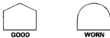
Fig. 190: Identifying Example Of Synchro Ring Teeth Courtesy of AMERICAN HONDA MOTOR CO., INC.
