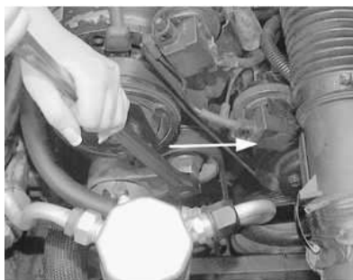
Fig. 2: Rotate the breaker bar in the tensioner toward the driver's side of the vehicle
