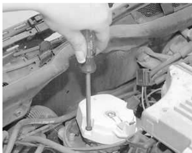
Fig. 10: . . . then pull the rotor straight up to remove it from the distributor
