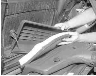
Fig. 5: Exploded view of the air cleaner assembly — 1984 vehicle shown
