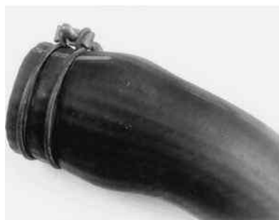
Fig. 3: A soft spongy hose (identifiable by the swollen section) will eventually burst and should be replaced
