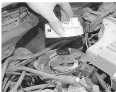
Fig. 10: . . . then pull the rotor straight up to remove it from the distributor
