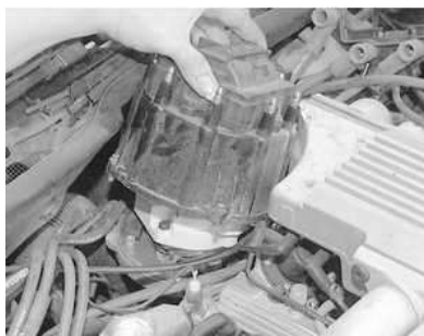
Fig. 8: Carefully lift the distributor cap up, and remove it from the vehicle
