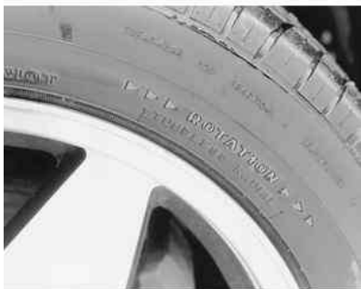
Fig. 2: Unidirectional tires are identifiable by sidewall arrows and/or the word "rotation"
