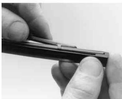
Fig. 6: To remove and install a Lexor( wiper blade refill, slip out the old insert and slide in a new one
