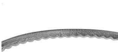
Fig. 2: An example of a healthy drive belt
