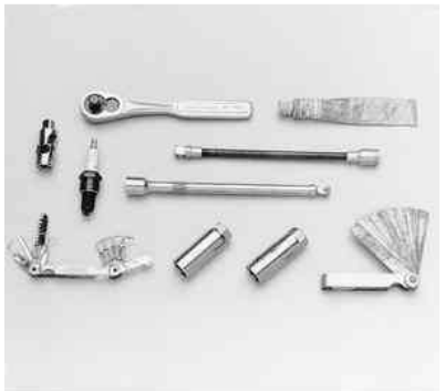
Fig. 2: A variety of tools and gauges are needed for spark plug service
