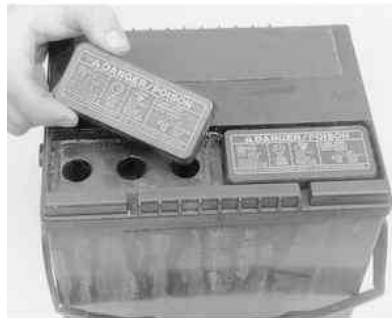
Fig. 1: On non-maintenance-free batteries, the fluid level can be checked through the case on translucent models; the cell caps must be removed on other models
