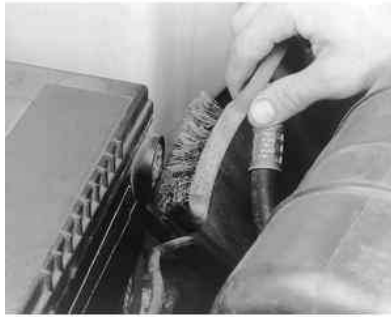
Fig. 5: The battery terminal can also be cleaned using a solution of baking soda and water
