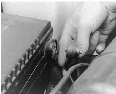
Fig. 2: . . . then disconnect the cable from the battery
