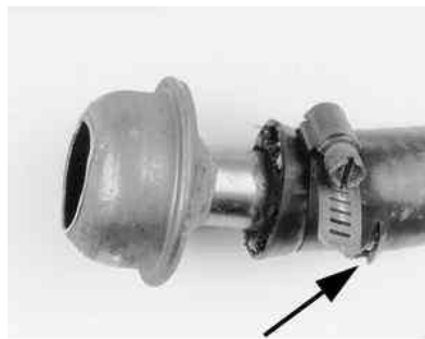
Fig. 2: A hose clamp that is too tight can cause older hoses to separate and tear on either side of the clamp
