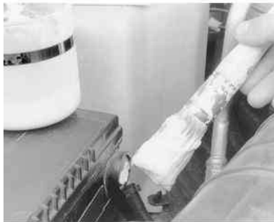
Fig. 5: The battery terminal can also be cleaned using a solution of baking soda and water
