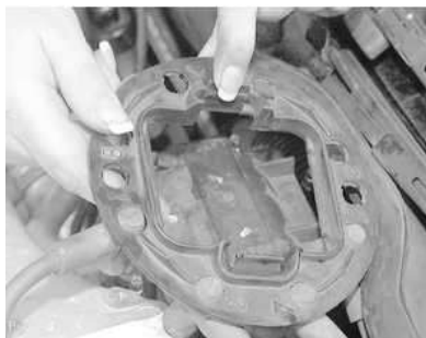
Fig. 3: Remove the distributor shield by pulling it up, off the spark plug wires
