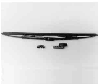
Fig. 6: To remove and install a Lexor( wiper blade refill, slip out the old insert and slide in a new one
