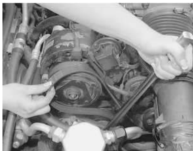
Fig. 3: Once the tension is relieved, you can remove the unrout the drive belt from the pulleys
