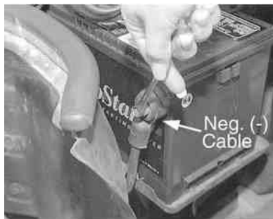
Fig. 5: ALWAYS disconnect the negative battery cable first!
