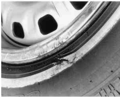
Fig. 2: Tires with deep cuts, or cuts which bulge, should be replaced immediately
