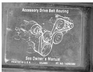
Fig. 6: There is usually an accessory drive belt routing label located in the engine compartment
