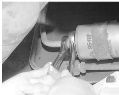
Fig. 2: ALWAYS use a back-up wrench when loosening the fuel feed pipes from the filter
