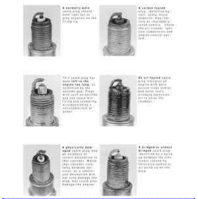
Fig. 1: Inspect the spark plug to determine engine running conditions
