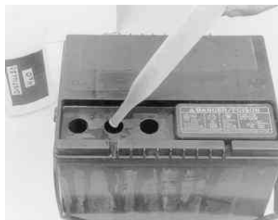
Fig. 2: If the fluid level is low, add only distilled water through the opening until the level is correct
