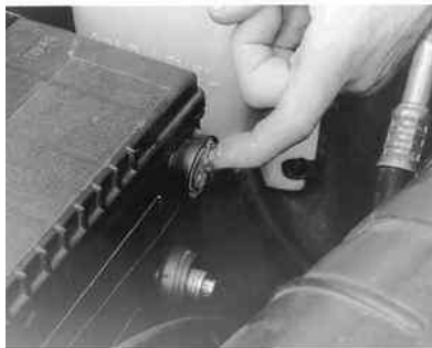
Fig. 6: Before connecting the cables, it's a good idea to coat the terminals with a small amount of dielectric grease
