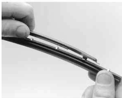
Fig. 9: . . . then the insert can be removed. After installing the replacement insert, bend the tab back
