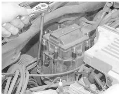
Fig. 7: On this 1986 vehicle, use a ratchet with a long extension to loosen the distributor cap bolts
