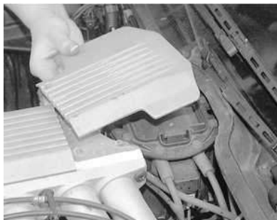
Fig. 2: Remove the plenum extension for access to the distributor cap
