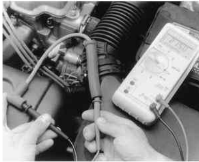
Fig. 1: Checking individual plug wire resistance with a digital ohmmeter
