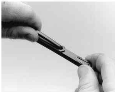
Fig. 10: The Tripledge® wiper blade insert is removed and installed using a securing clip
