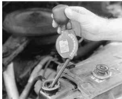
Fig. 1: A coolant tester can be used to determine the freezing and boiling levels of the coolant in your vehicle
