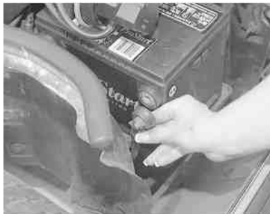
Fig. 6: Make sure to place the cable out of the way so it doesn't accidentally contact the terminal
