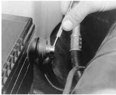
Fig. 1: Loosen the battery cable retaining nut . . .
