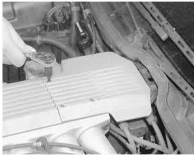
Fig. 1: Unfasten the plenum extension Torx® retaining screws
