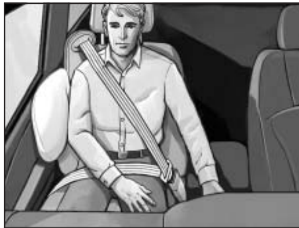
The right front passenger's side impact airbag is in the side of the passenger's seatback closest to the door.
