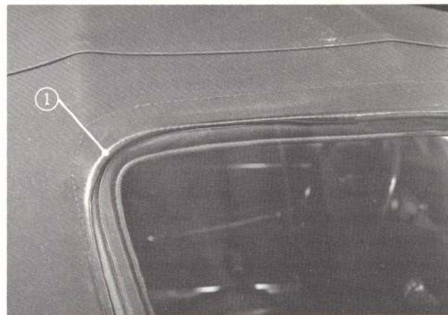
Window too high, pinching top piping.
