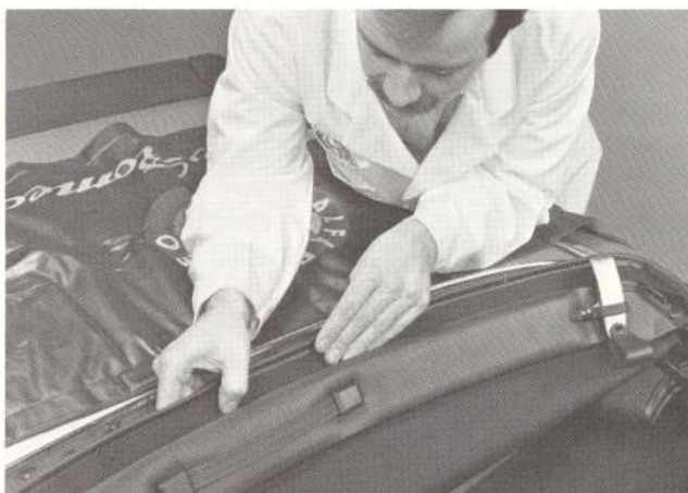
Applying top to frame front edge.
