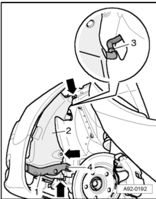
Fig. 247: Removing Bottom Section Of Reservoir Courtesy of VOLKSWAGEN UNITED STATES, INC.
