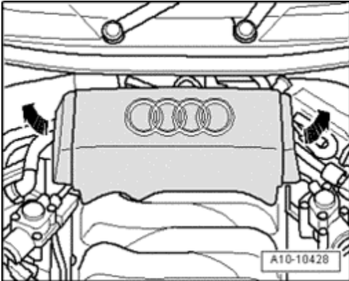
Fig. 87: Pulling Rear Engine Cover
