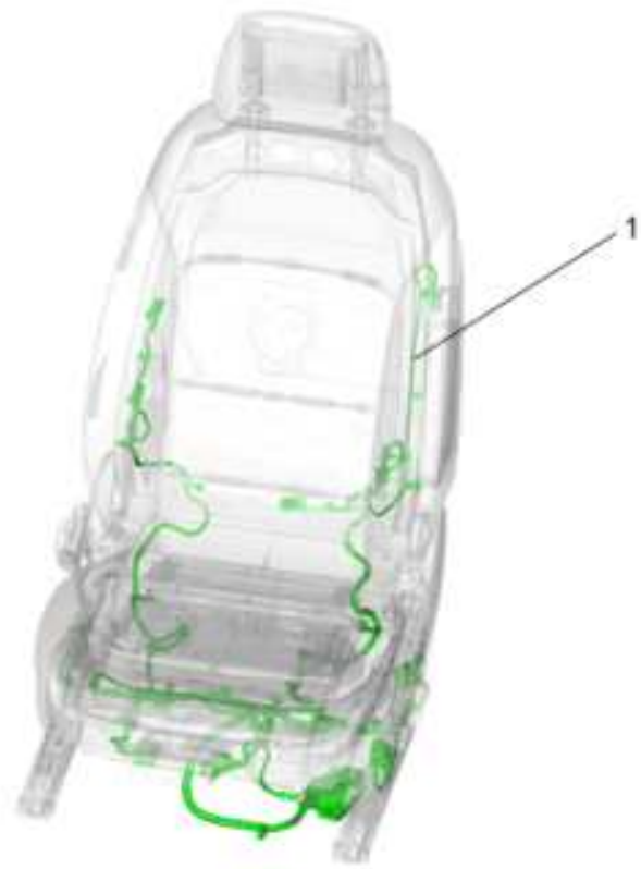
Fig. 23: Front Seat Wiring Harness Courtesy of GENERAL MOTORS COMPANY
