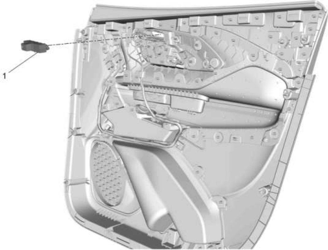
Fig. 15: Front Seat Adjuster Memory Switch (Terrain) Courtesy of GENERAL MOTORS COMPANY
