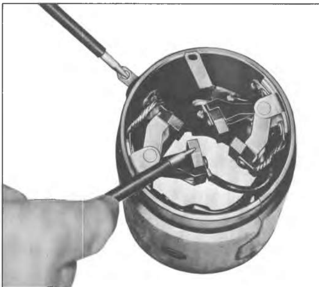
Fig. 6D-6S--Field Coil Open Circuit Test
