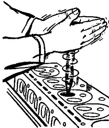
Lapping the valve and seat by hand—typical
