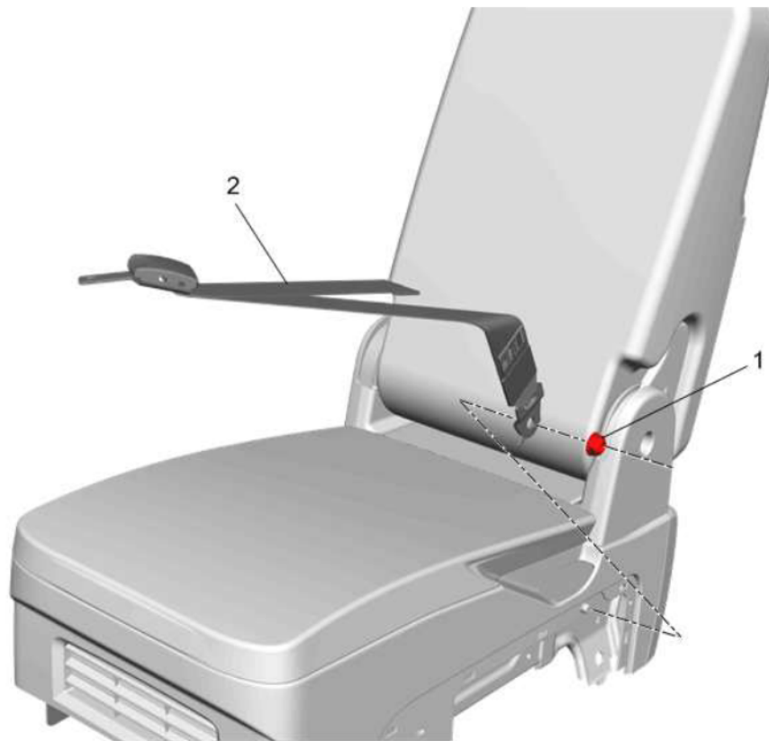
Fig. 5: Front Seat Belt Latch (HP5) Courtesy of GENERAL MOTORS COMPANY
