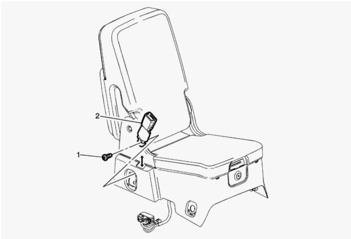
Fig. 6: Front Center Seat Belt Buckle (with AZ3) Courtesy of GENERAL MOTORS COMPANY
