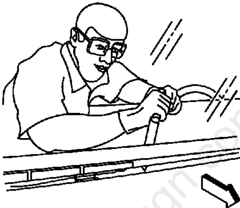
Fig. 26: Separating Bottom Of Window Courtesy of GENERAL MOTORS COMPANY
