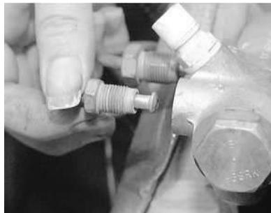
Fig. 3: Pull the brake lines from the side of the master cylinder, then plug the holes to avoid contaminating the system
