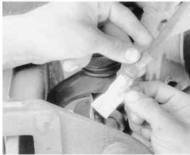
Fig. 9: Tape or plug the line to prevent contamination
