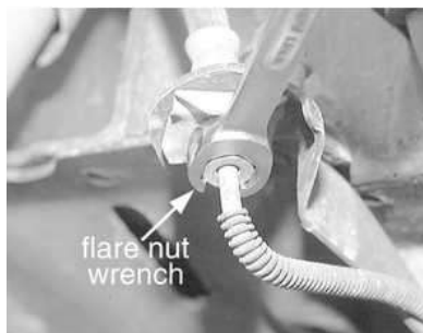
Fig. 3: When possible, use a flare nut wrench to loosen brake lines
