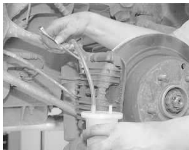
Fig. 2: With a hose over the end of the bleeder valve, and the other end submerged in clean brake fluid, open the valve to bleed the system
