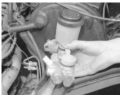
Fig. 5: Unfasten the retaining nuts, then pull the master cylinder off the power booster studs
