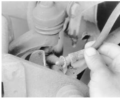
Fig. 9: Tape or plug the line to prevent contamination
