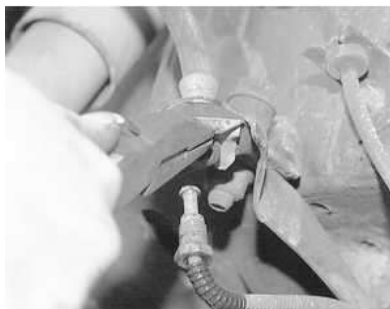
Fig. 7: Remove any routing clips retaining the brake line that is being removed
