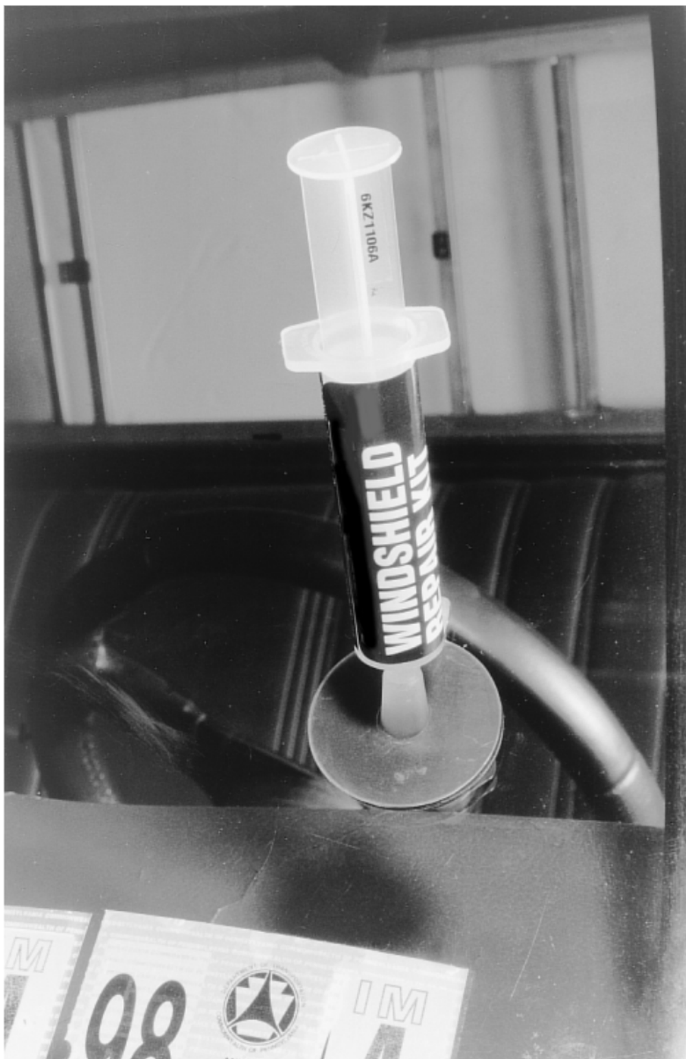
Fig. 2: Most kits use a self-stick applicator and syringe to inject the adhesive into the chip or crack
