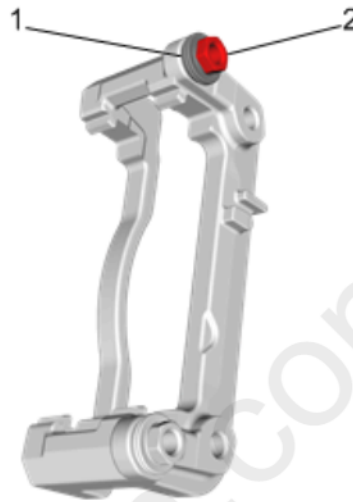
Fig. 11: Upper Guide Pin Seal And Guide Pin Seal Courtesy of GENERAL MOTORS COMPANY
