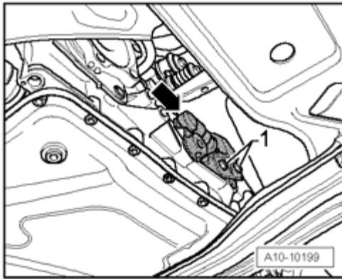
Fig. 42: Removing Bolts For Support Bracket From Transmission & Disengaging Selector Lever Cable Courtesy of VOLKSWAGEN UNITED STATES, INC.
