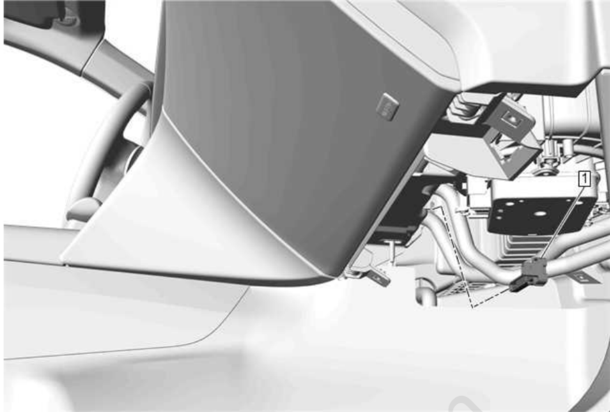
Fig. 73: Evaporator Air Temperature Sensor Courtesy of GENERAL MOTORS COMPANY
