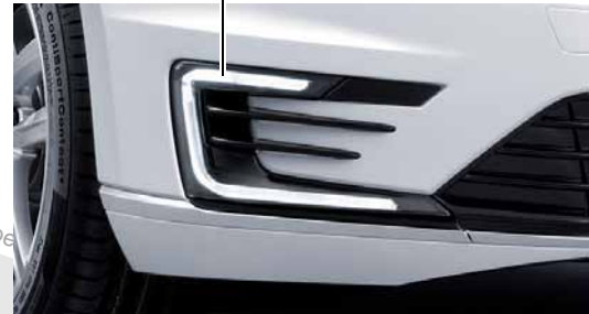
Daytime running light 4 LEDs (3 W each)
