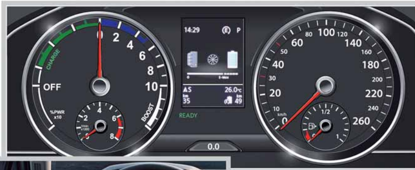
Dash panel insert with GTE-specific gauges
