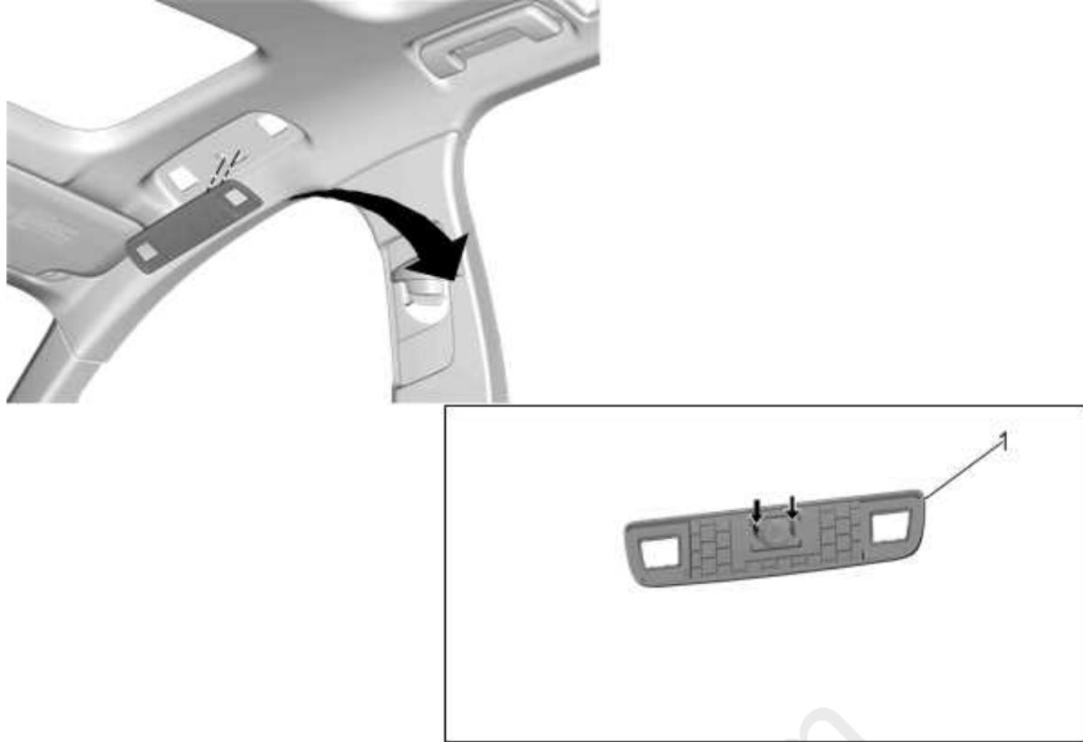
Fig. 11: Active Noise Cancellation Microphone Grille (Front) Courtesy of GENERAL MOTORS COMPANY
