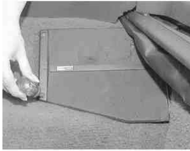
Fig. 4: Lift the speaker grille off to get to the speaker underneath
