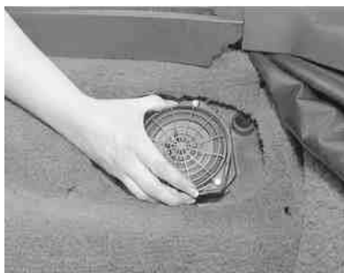
Fig. 6: After the screws are loosened or removed, as applicable, carefully lift the speaker up, detach the connector and remove it from the vehicle
