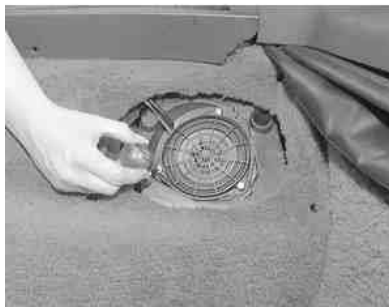
Fig. 5: The speaker is usually secured with 3 or 4 retaining screws
