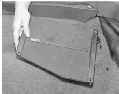
Fig. 4: Lift the speaker grille off to get to the speaker underneath
