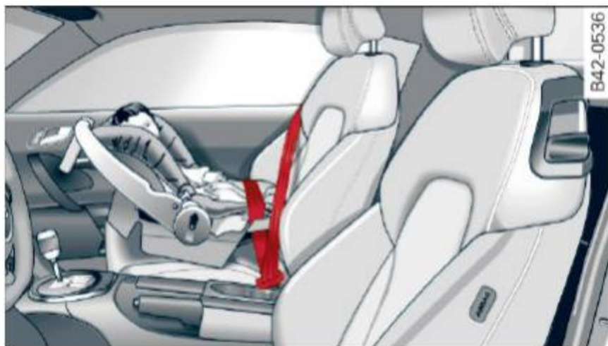
Fig. 98 Rearward-facing infant seat, properly installed on the passenger seat
