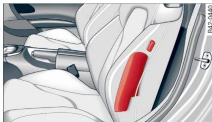
Fig. 96 Side airbag location in the driver's seat
