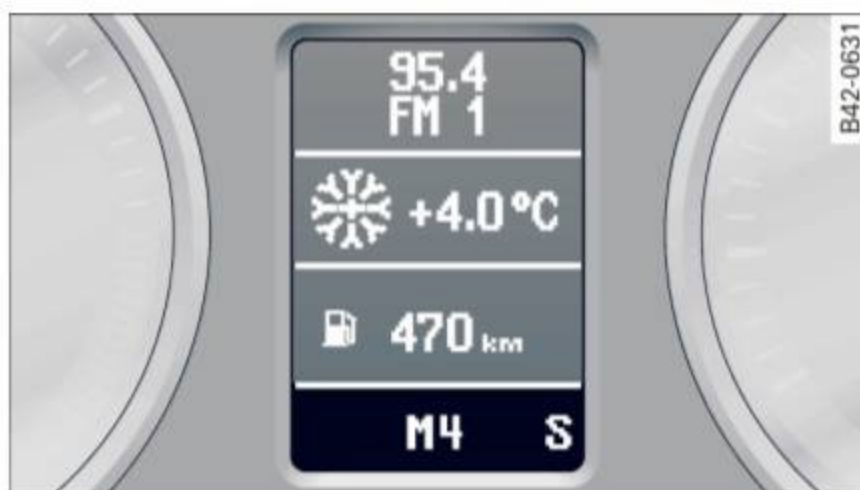
Fig. 64 Display: selected gears
