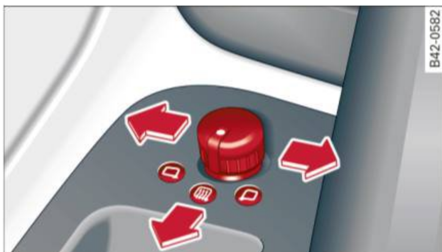
Fig. 40 Forward section of driver's armrest: power mirror controls
