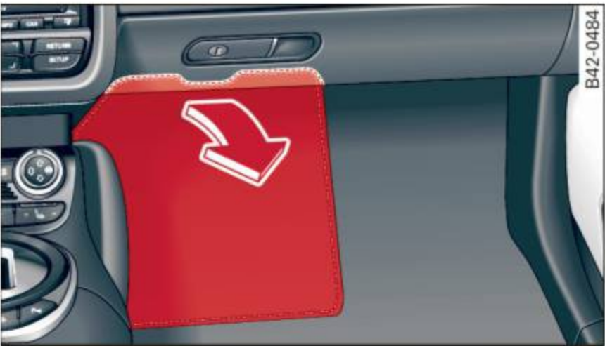
Fig. 139 Passenger's side wheel well: Foot rest with fuse arrangement
