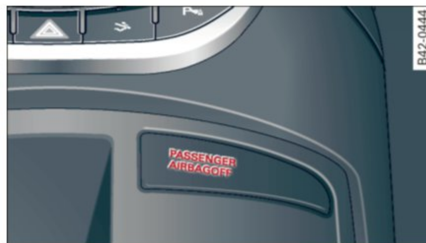
Fig. 93 Section from the instrument panel: PASSENGER AIR BAG OFF light
