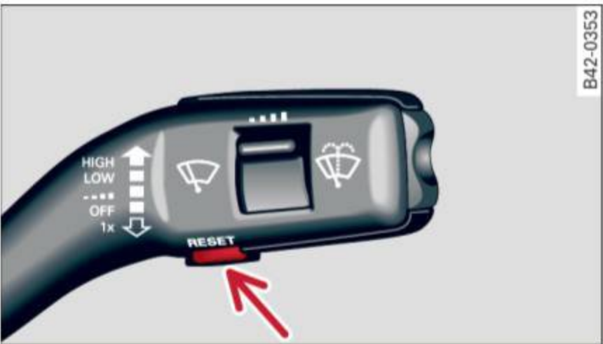
Fig. 7 Wiper lever: controls for the menu display
