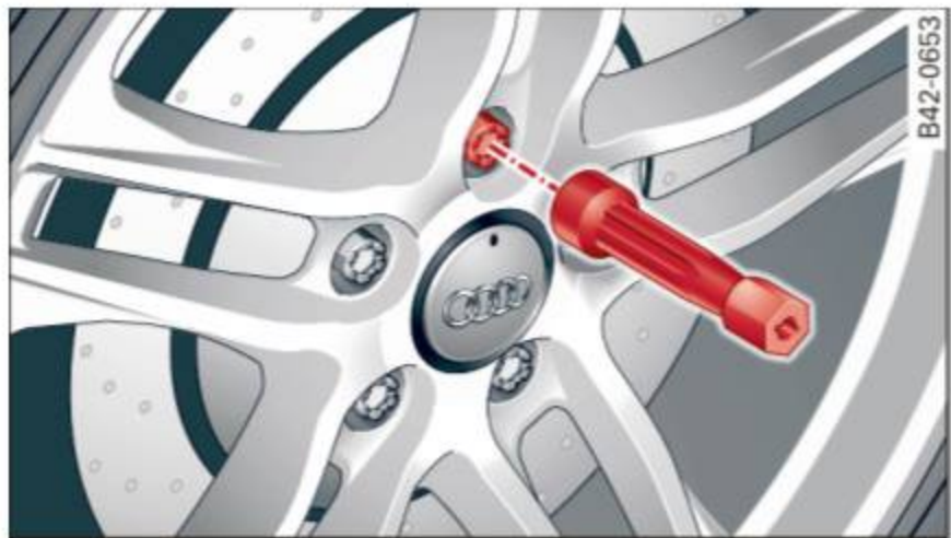
Fig. 134 Wheel change: using the screwdriver handle (with the blade removed) to turn the bolts
