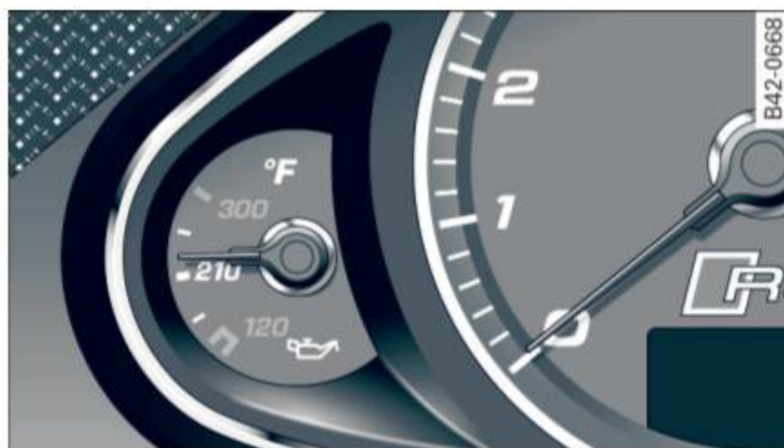
Fig. 112 Instrument cluster: Engine oil temperature display
