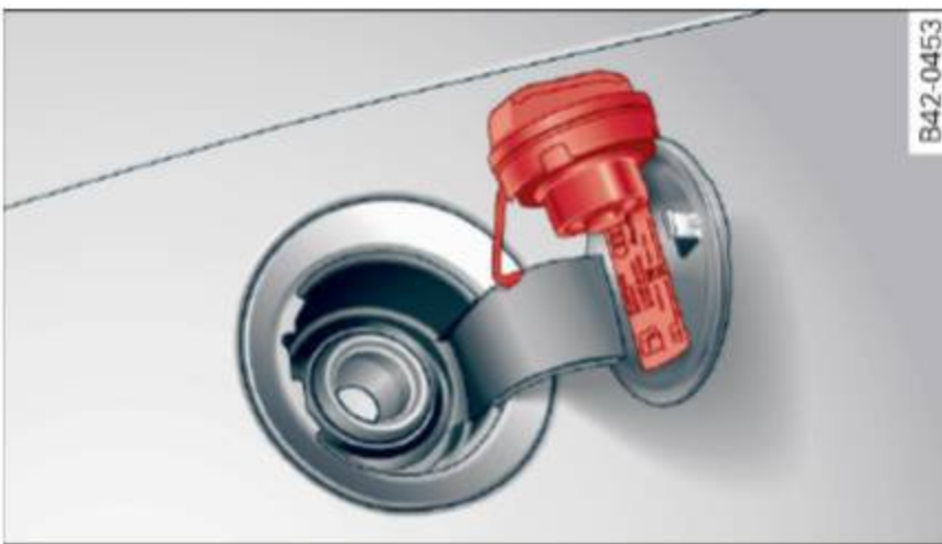
Fig. 106 Fuel cap hooked on the opened fuel filler flap
