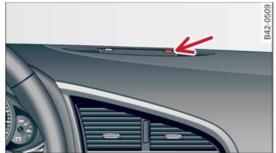
Fig. 30 Diode position in the instrument panel
