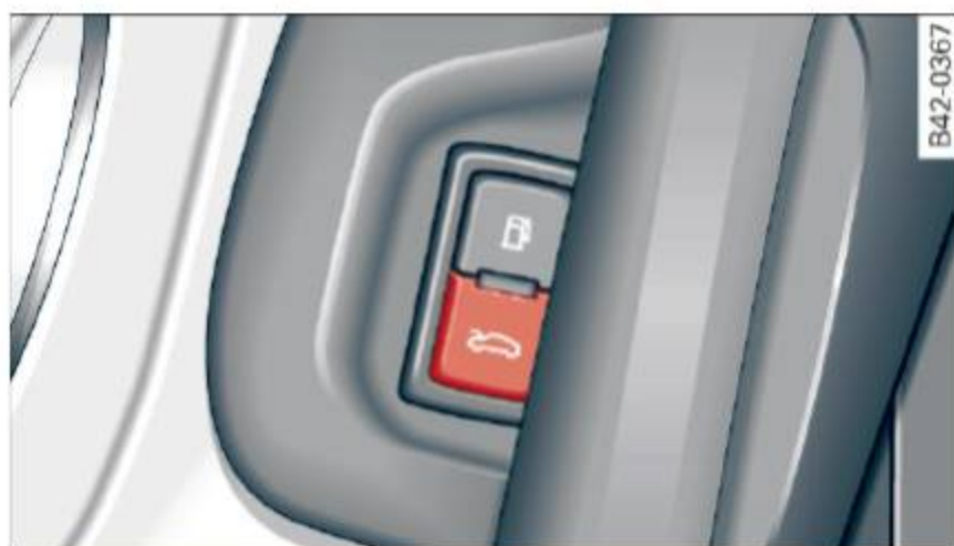
Fig. 27 Drivers door: remote front lid release
