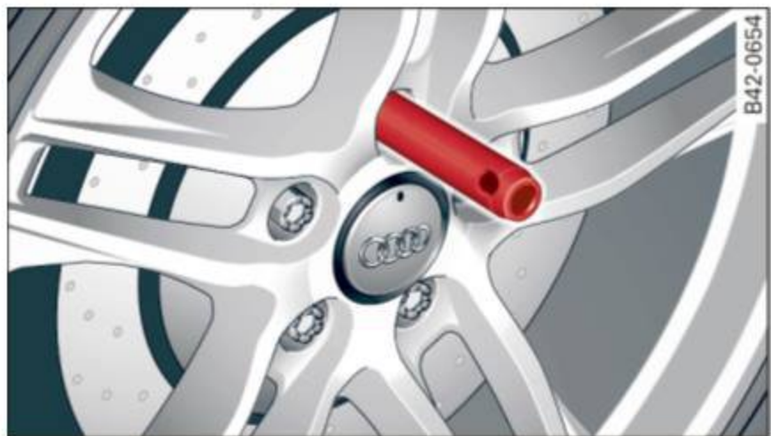
Fig. 135 Wheel change: alignment pin inside the top hole
