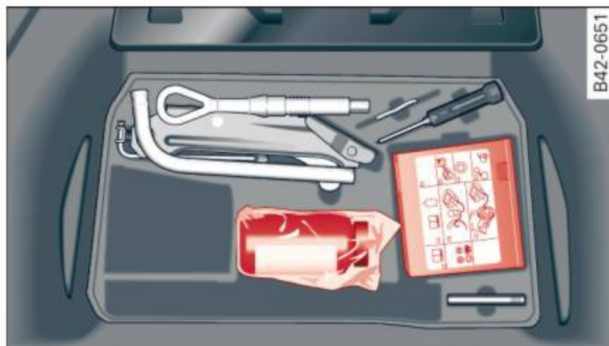
Fig. 128 Tire Mobility System under luggage compartment floor
