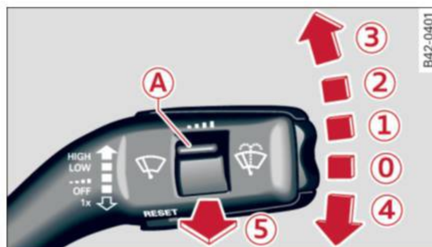
Fig. 43 Wiper lever: windshield wiper lever positions
