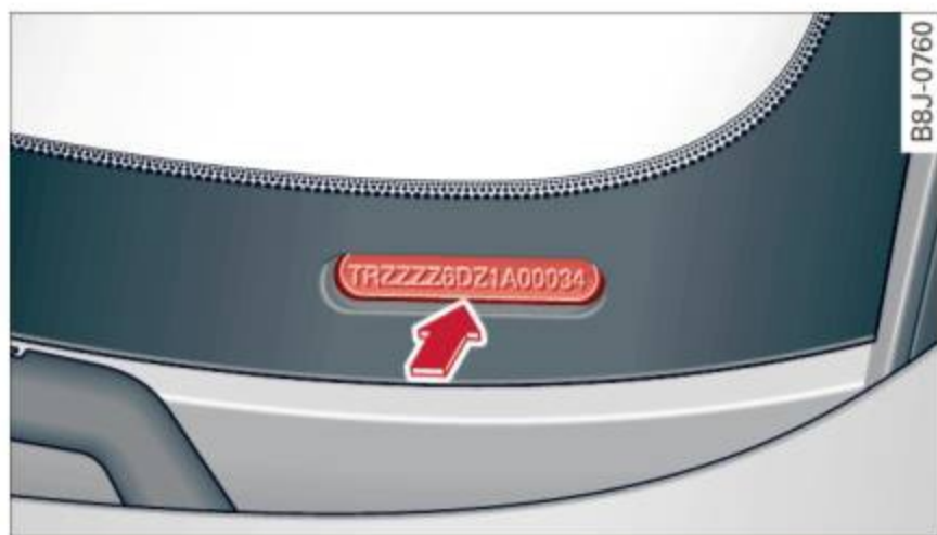
Fig. 141 Vehicle Identification Number (VIN) plate: location on driver's side dash panel
