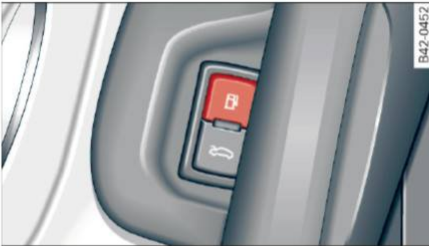
Fig. 105 Driver's door: Unlocking fuel filler flap
