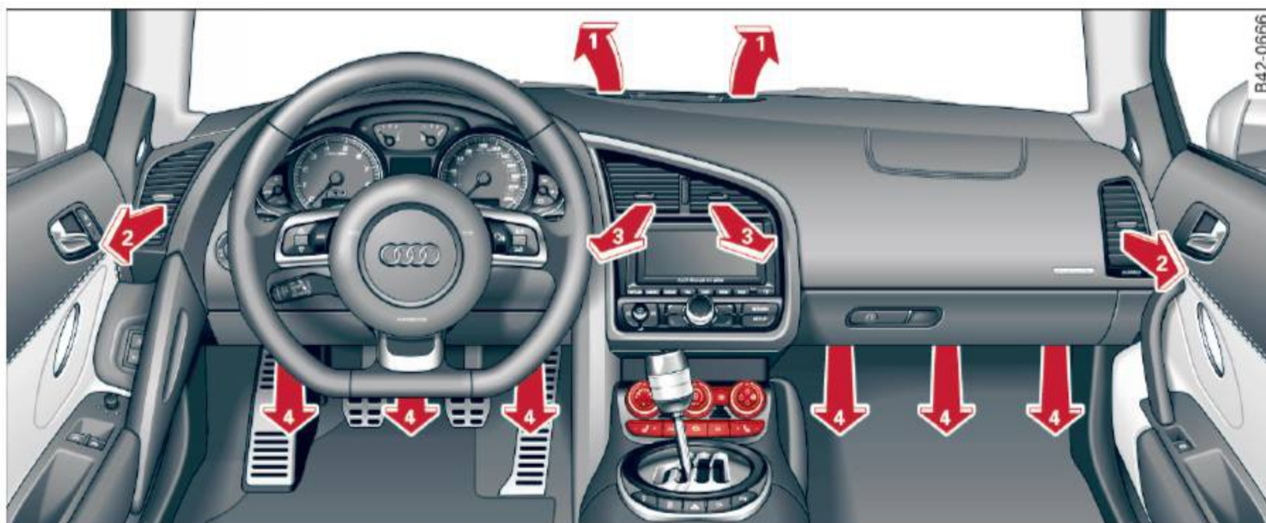
Fig. 54 Instrument panel: Location of air vents
