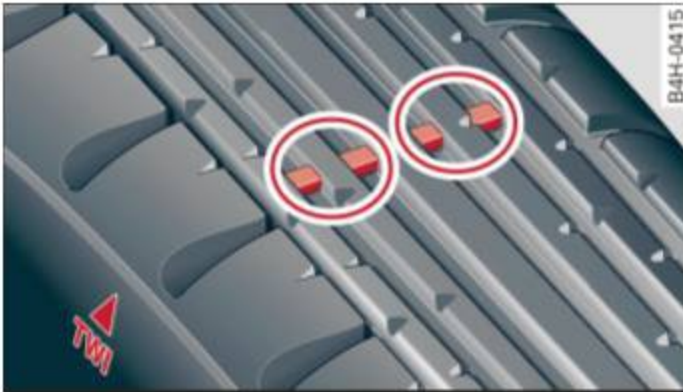
Fig. 124 Tire tread: tread wear indicators (TWI)
