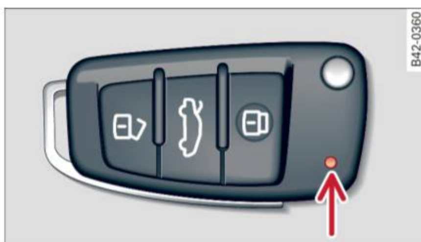
Fig. 21 Remote master key: Indicator light
