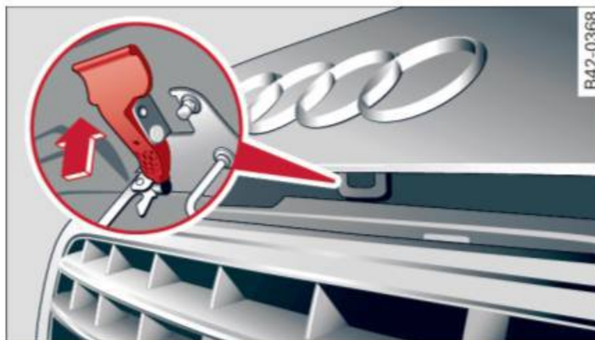
Fig. 28 Release lever under the front lid
