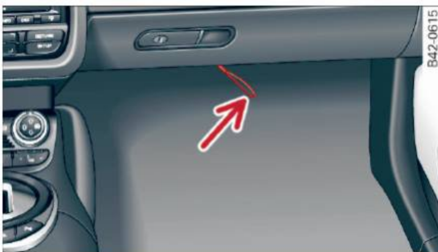
Fig. 29 Section: Emergency release
