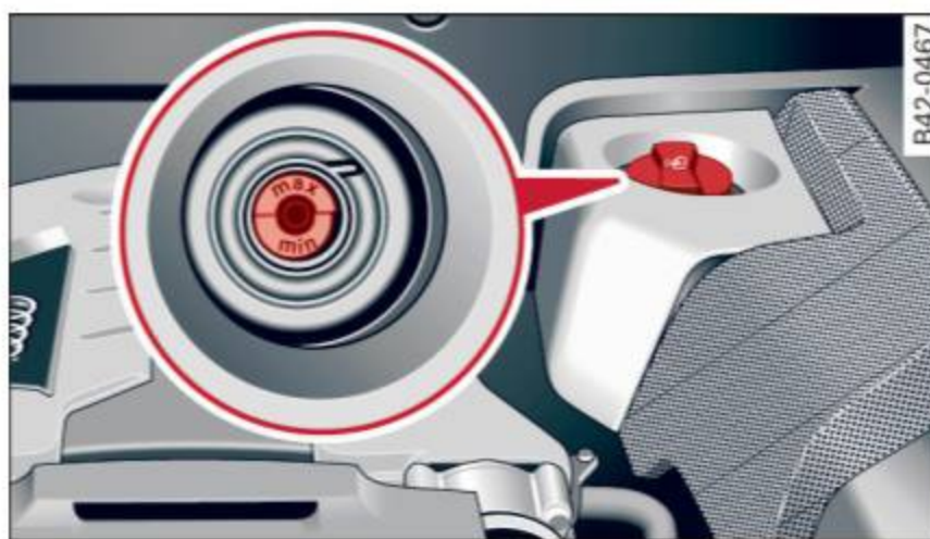
Fig. 118 Engine compartment: coolant expansion tank
