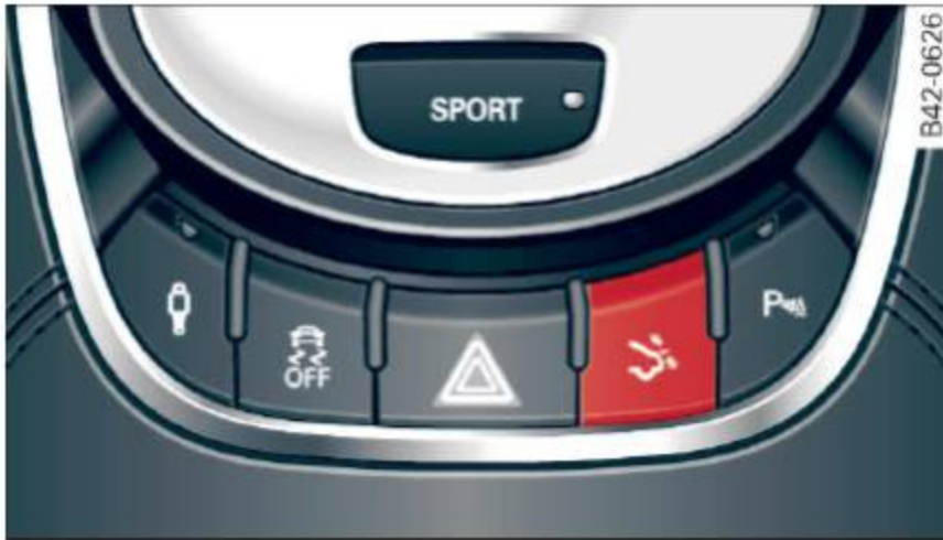
Fig. 104 Switch for rear spoiler
