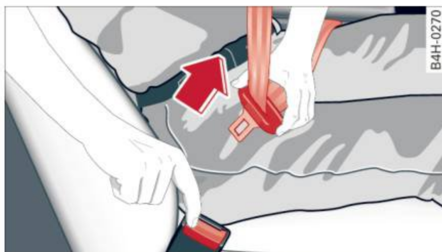
Fig. 89 Releasing the tongue from the buckle
