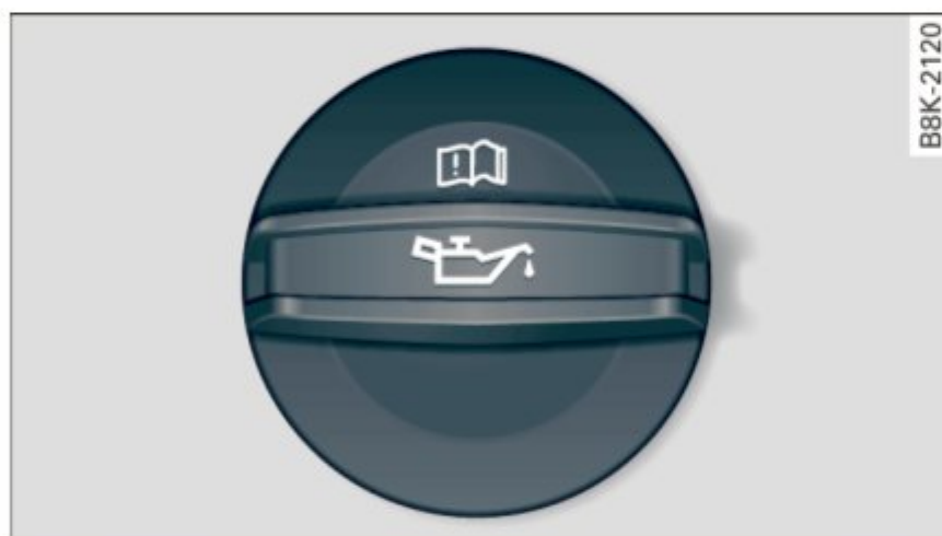
Fig. 117 Engine compartment: cover on the engine oil filler neck
