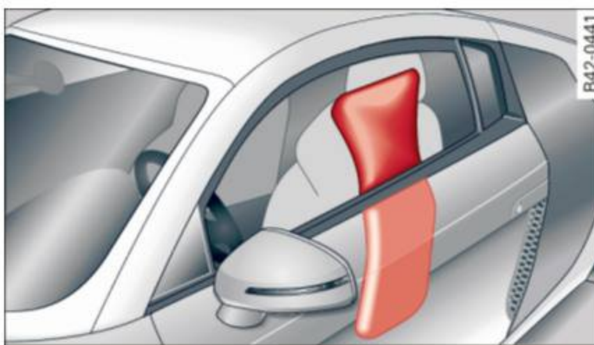
Fig. 97 Inflated side airbags on left side of vehicle
