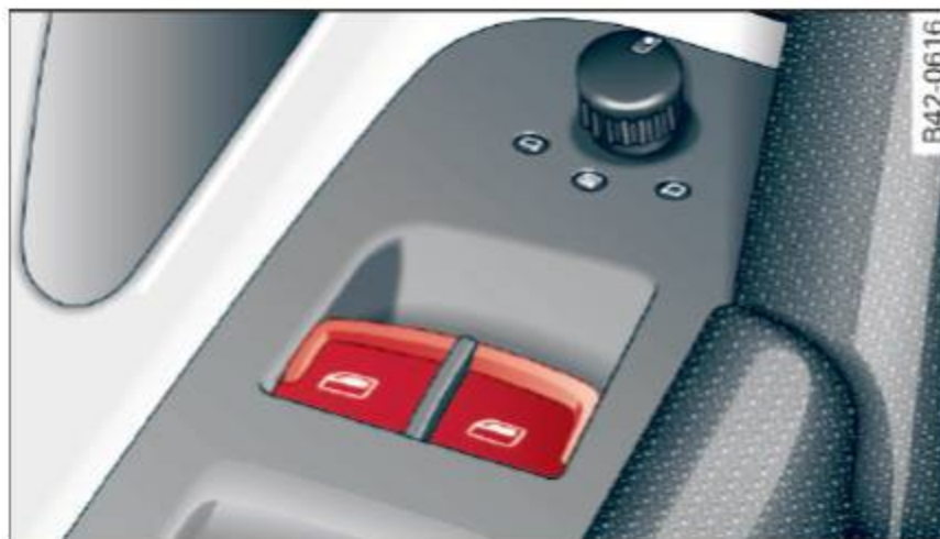
Fig. 31 Driver's door: power window switches
