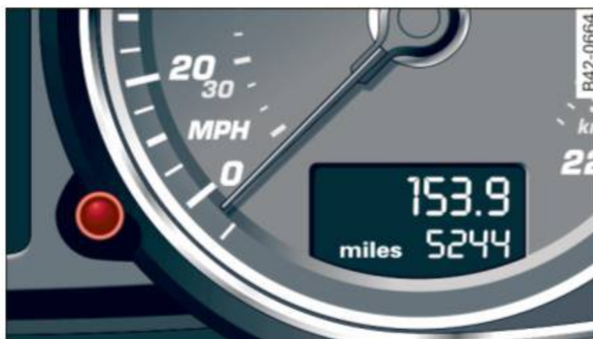
Fig. 5 Speedometer close-up: odometer display
