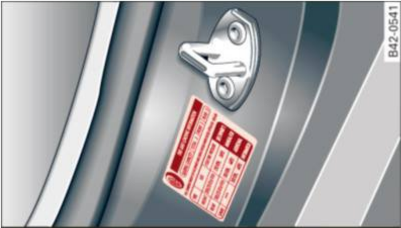
Fig. 122 Tire pressure label: located on driver's side B-pillar
