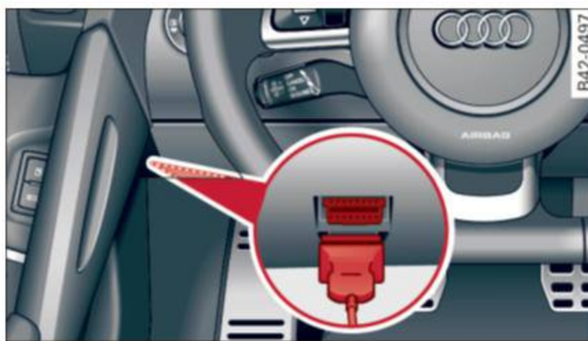
Fig. 19 Location of Data Link Connector (DLC)
