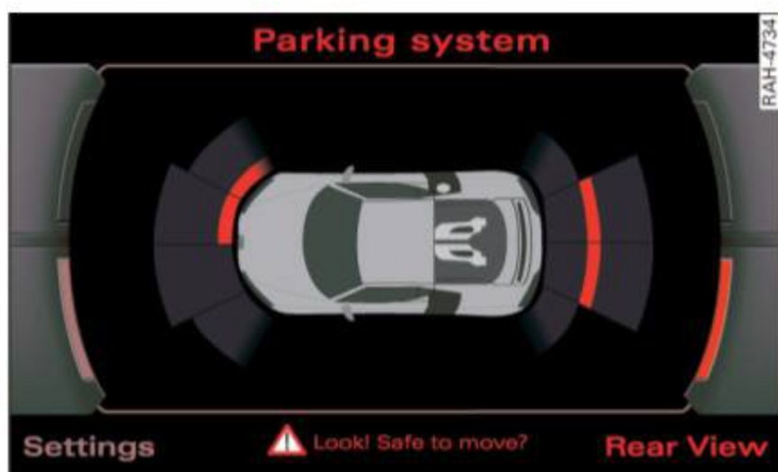
Fig. 73 Navigation system display: visual distance display
