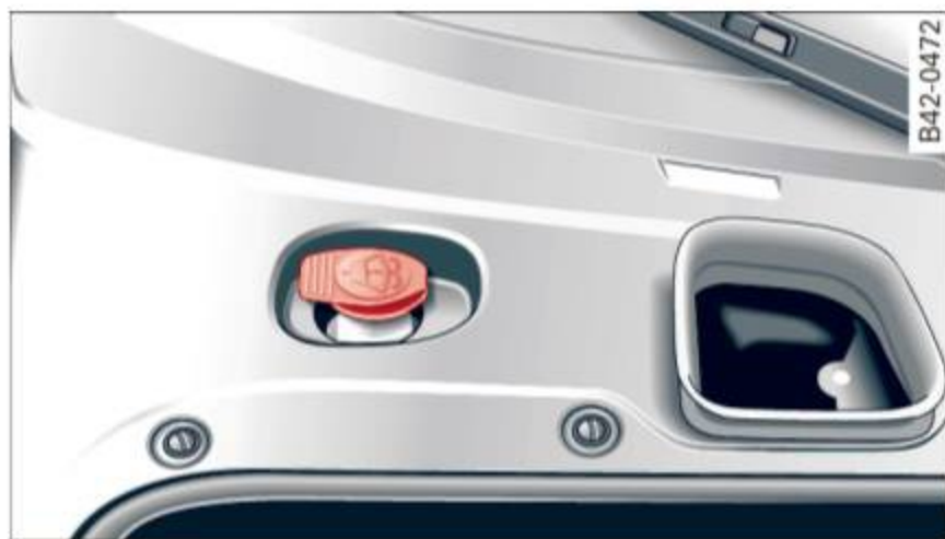
Fig. 121 Luggage compartment: Windshield washer fluid reservoir
