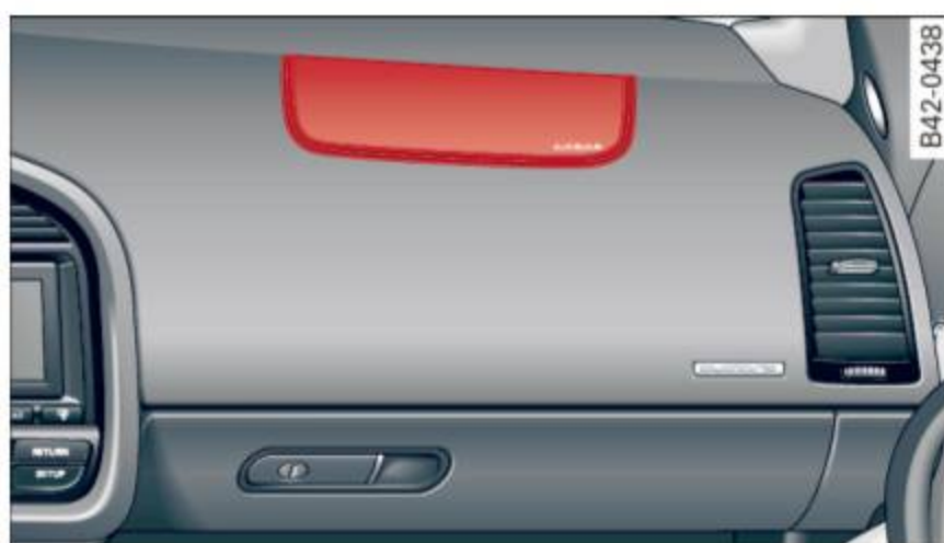
Fig. 91 Location of front passenger's airbag: in the instrument panel
