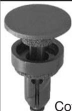
18119 (91502-SP0-003) Black Nylon Front & Rear Bumper Push-Type Retainer Head Diameter: 20mm Stem Length: 25mm Fits Into 10mm Hole Honda 1990-On
