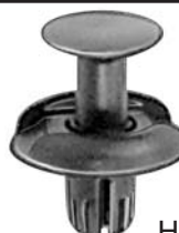
19186 (90657-SB0-003) Black Nylon Front Bumper Cover Push-Type Retainer Head Diameter: 11mm Stem Length: 10mm Fits Into 8mm Hole Acura Legend, Honda Accord & Odyssey 1991-On
