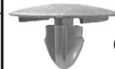
19113 (90467-08124) Black Nylon Hood Insulation Retainer Head Diameter: 25mm Stem Diameter: 8mm Stem Length: 12mm Toyota Supra 1993-On Lexus 1994-89 UNIT PACKAGE: 15
