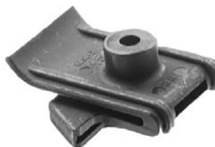
19735 (63848-35F00) Black Nylon Fender Clip "U" Nut #10 Screw Size 20mm Wide 32mm Long Panel Range: Up To 2mm Center Of Hole To Edge: 8mm Maxima & 240SX 1994 - On
