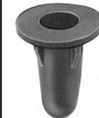
19013 (90467-07059-22) Black Nylon Rear Door Trim & Luggage Compartment Door Push-Type Retainer Head Diameter: 15mm Stem Length: 10mm Fits Into 7mm Hole Camry & Celica 1990-On
