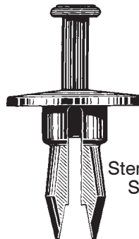
12757 (5973400) Black Nylon Fascia Retainer Stem :3/4"/ Head Dia: 1" Shoulder Length: 1/8" Fits Into 1/2" Hole GM 1979-On
