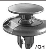
19547 (91508-S50-003) Black Nylon Cowl Top Retainer Head Diameter: 17mm Stem Length: 13mm (Exc. Pin) Fits Into 9mm Hole Accord & Odyssey 1998 - On
