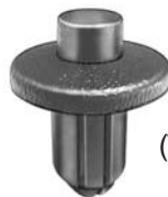
19739 (90467-09127) Black Nylon Bumper Cover Push-Type Retainer Head Diameter: 20mm Stem Length: 26mm Fits Into 9mm Hole Avalon, Camry, Corolla & Solara 1998 - On
