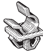
14732 (53455-14020) Nylon Hood Prop Rod Clip Holds 8mm Dia. Rod Snaps Into 14mm Hole
