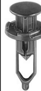
18873 (52161-16010) Black Nylon Rear Bumper Cover Push-Type Retainer Head Diameter: 18mm Stem Length: 28mm Fits Into 9mm Hole Tercel 1988-On
