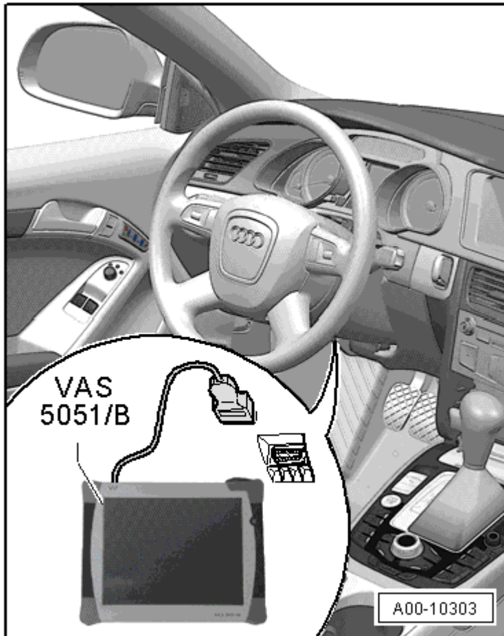
Fig. 51: Connecting Diagnostic Cable VAS 5051/5A To Diagnostic Connector
