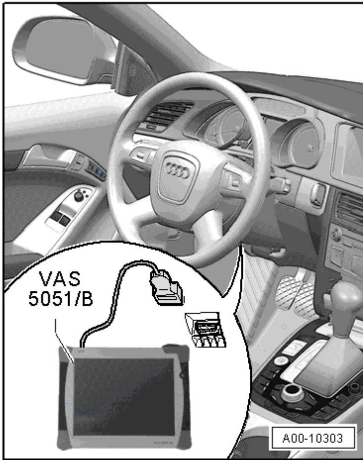
Fig. 151: Connecting Diagnostic Cable VAS 5051/5A To Diagnostic Connector Courtesy of AUDI OF AMERICA, LLC
