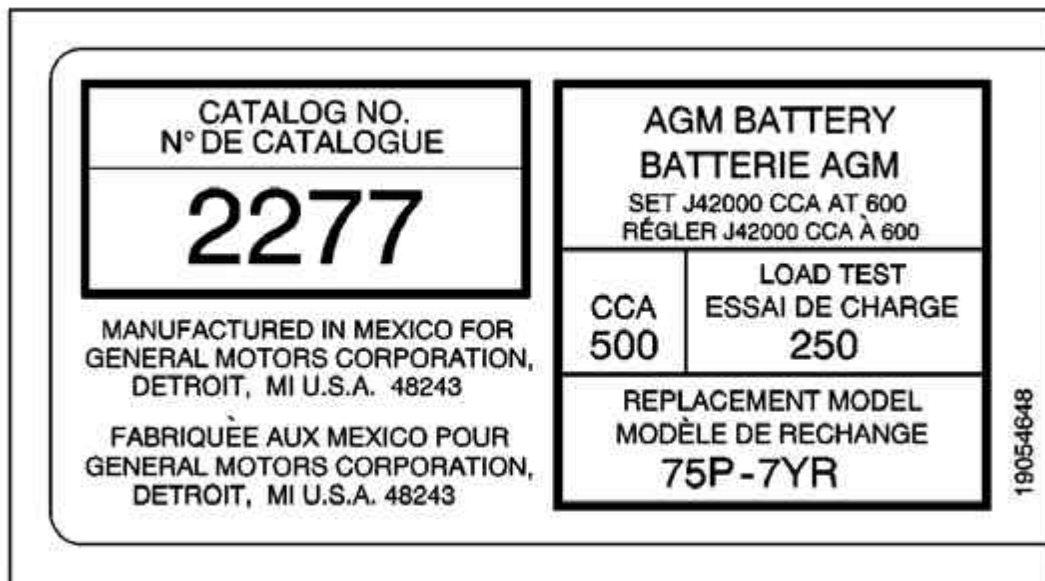
Fig. 119: Identifying Battery Rating Courtesy of GENERAL MOTORS CORP.
