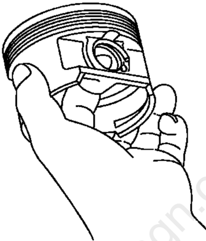
Fig. 148: View Of Retaining Clip In Pin Bore Groove Courtesy of GENERAL MOTORS COMPANY
