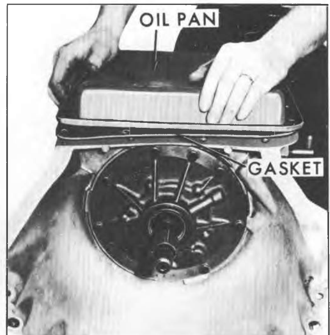
Fig. 7A-12B--Removing Transmission Oil Pan
