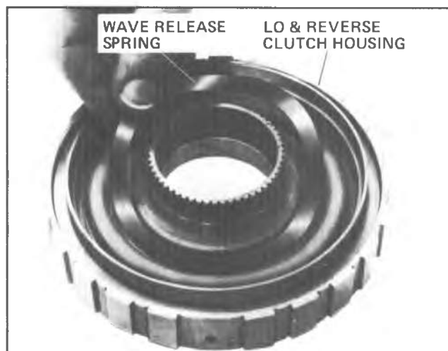
Fig. 7A-74A--Removing or Installing Low and Reverse Clutch Wave Release Springs
