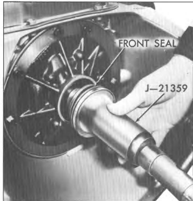
Fig. 7A-168C—Installing Pump Seal
