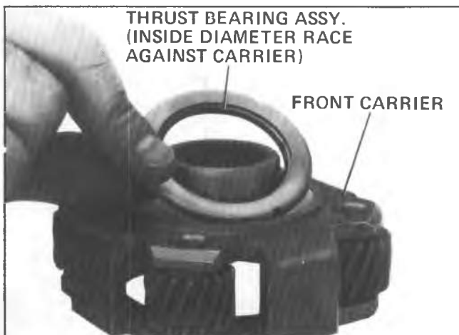
Fig. 7A-91A--Installing Thrust Bearing Assembly Onto Front Carrier
