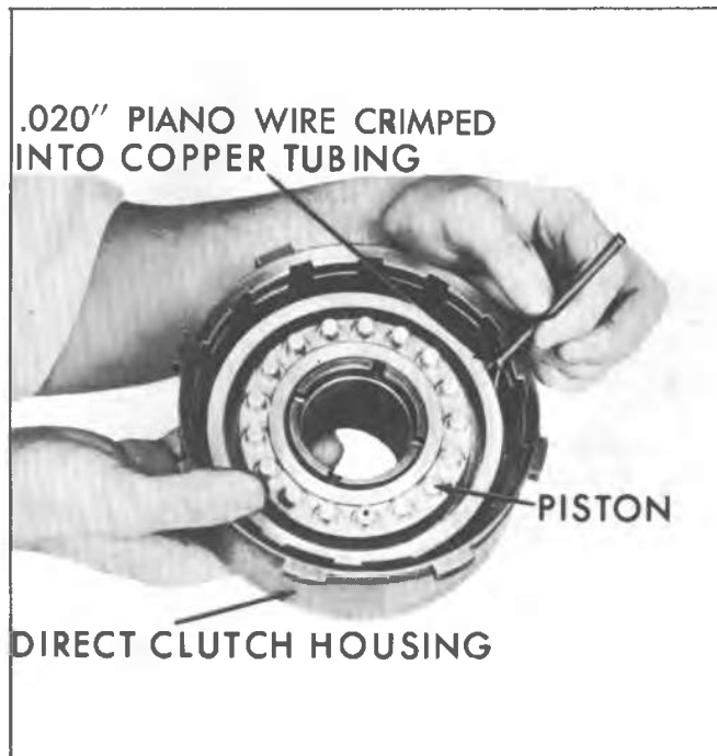
Fig. 7A-78B--Installing Direct Clutch Piston
