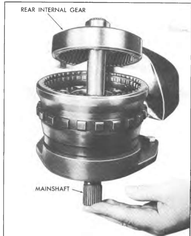
Fig. 7A-51C--Removing Rear Internal Gear and Mainshaft
