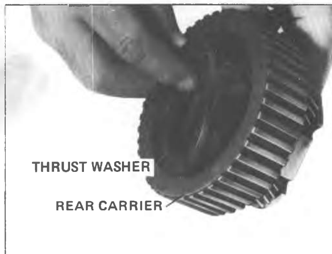
Fig. 7A-64A--Installing Thrust Washer Into Rear Carrier
