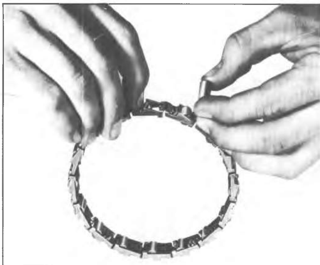
Fig. 7A-149C--Installing Roller into Roller Clutch Cage
