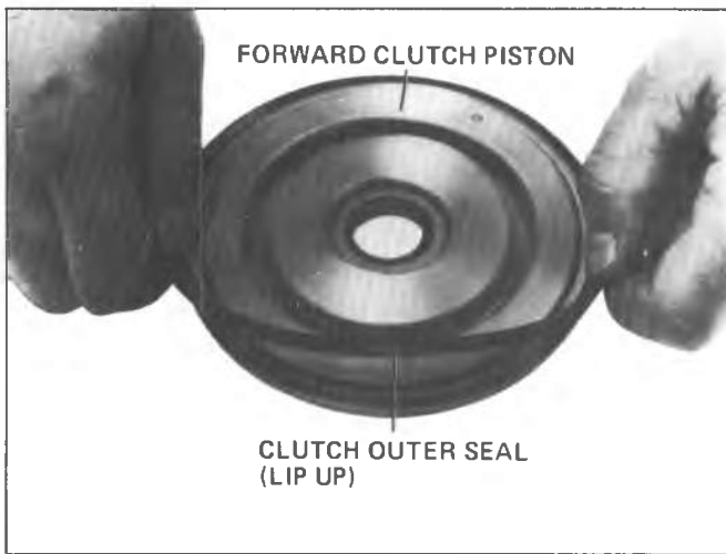
Fig. 7A-114A--Removing or Installing Outer Piston Seal
