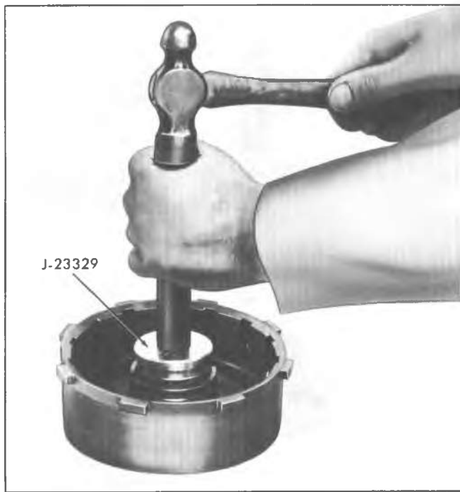
Fig. 7A-106B--Installing Direct Clutch Drum Bushing
