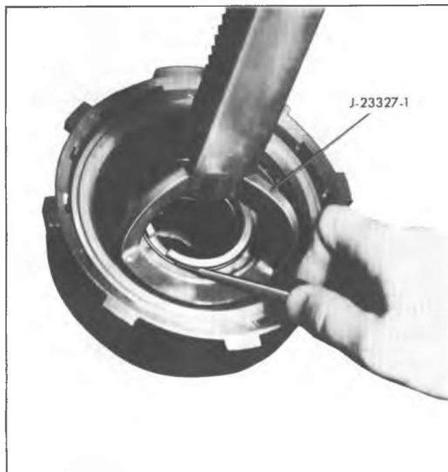
Fig. 7A-76B--Removing Direct Clutch Outer and Inner Seals
