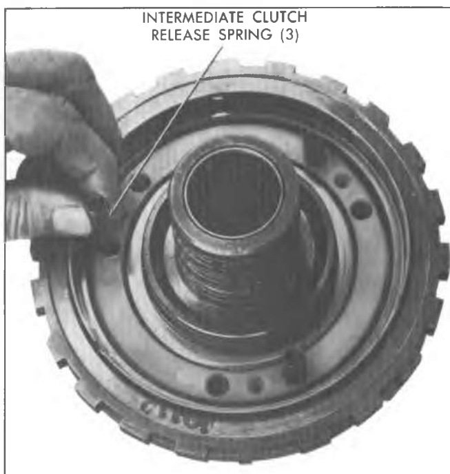
Fig. 7A-115C--Removing Clutch Release Springs
