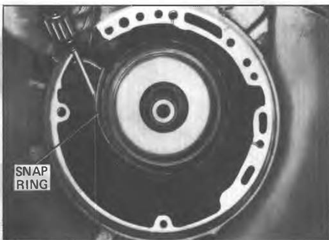
Fig. 7A-34A--Removing Low and Reverse Housing to Case Snap Ring
