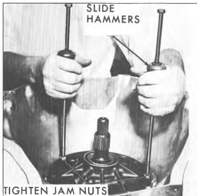
Fig. 7A-30B--Removing Pump from Case
