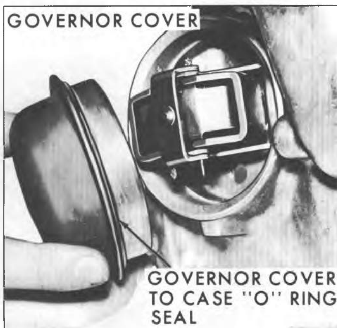
Fig. 7A-10B--Governor Cover and "O" Ring Seal
