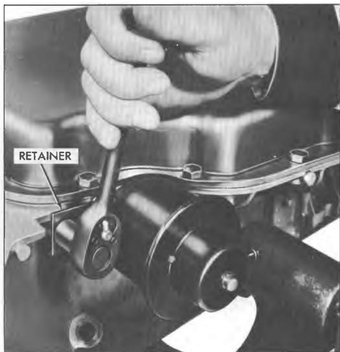
Fig. 7A-3C--Removing Modulator Retainer
