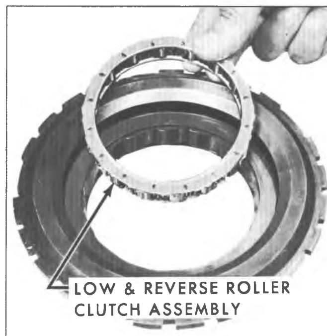
Fig. 7A-96B--Removing Overrun Roller Clutch Assembly
