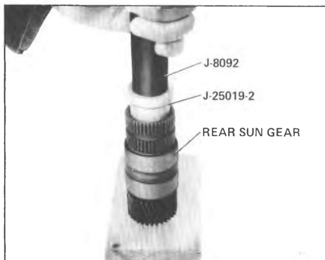
Fig. 7A-181A--Installing Rear Sun Gear Bushing
