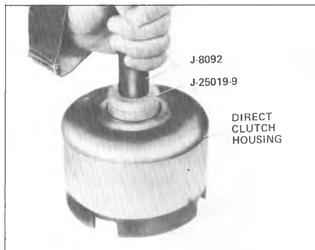
Fig. 7A-175A--Installing Direct Clutch Housing Bushing - Front
