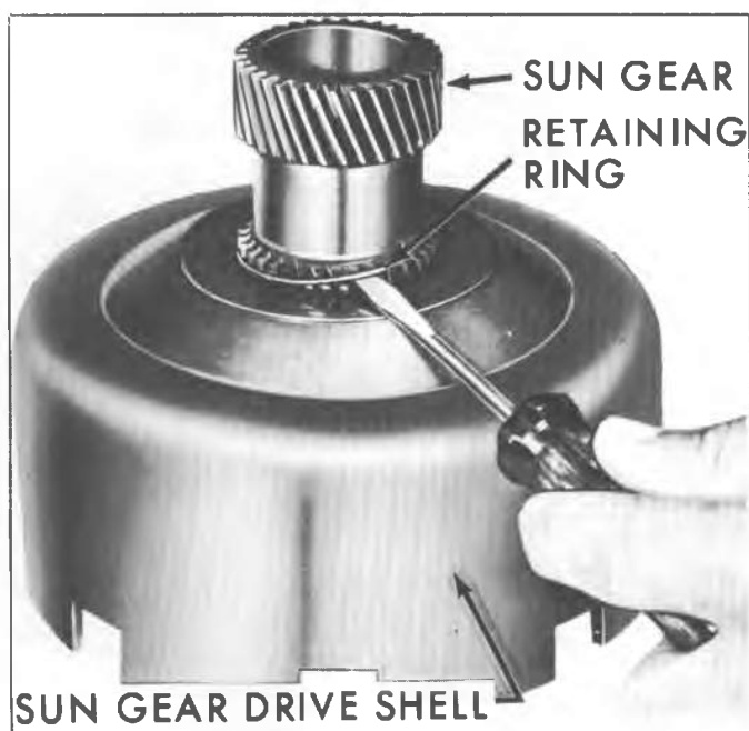
Fig. 7A-90B-Removing Sun Gear Drive Shell Rear Retaining Ring
