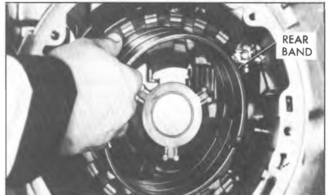
Fig. 7A-156C--Installing Rear Band
