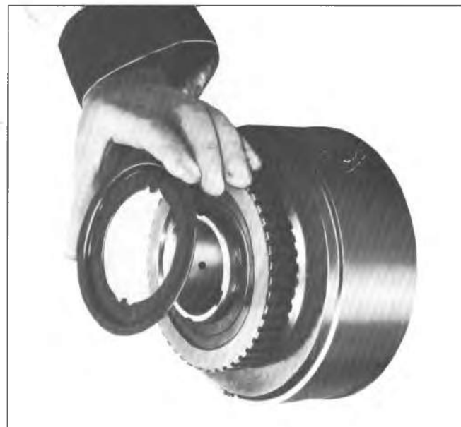
Fig. 7A-109C--Installing Intermediate Clutch Retainer
