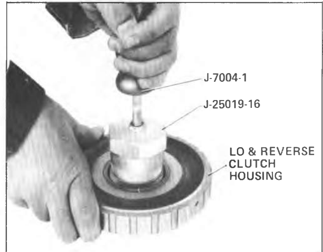
Fig. 7A-182A--Removing Lo and Reverse Clutch Housing Bushing
