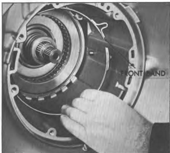
Fig. 7A-163C--Installing Front Band
