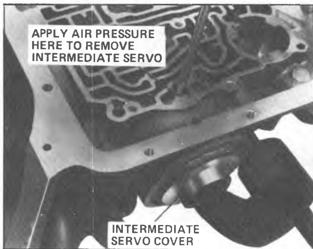
Fig. 7A-13A--Removing Intermediate Servo
