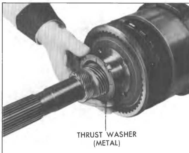
Fig. 7A-152C--Installing Case to Output Shaft Thrust Washer
