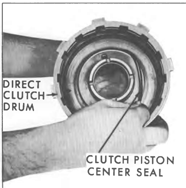
Fig. 7A-77B--Removing Direct Clutch Piston Center Seal
