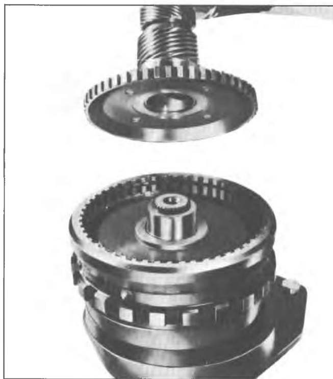
Fig. 7A-145C--Installing Output Shaft
