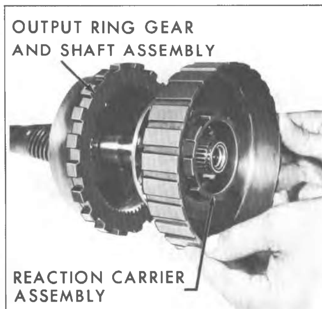
Fig. 7A-44B--Removing Reaction Carrier Assembly
