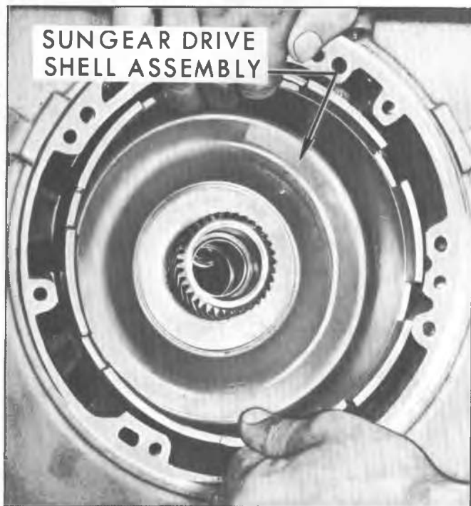
Fig. 7A-41B--Removing Sun Gear Drive Shell
