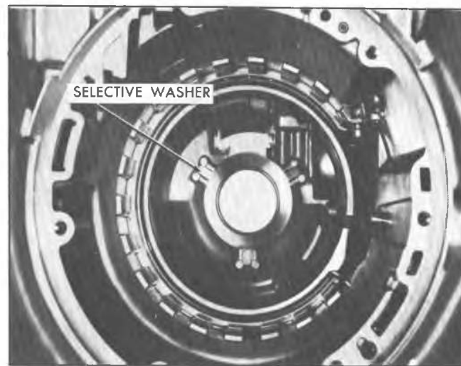
Fig. 7A-43C--Removing Selective Washer
