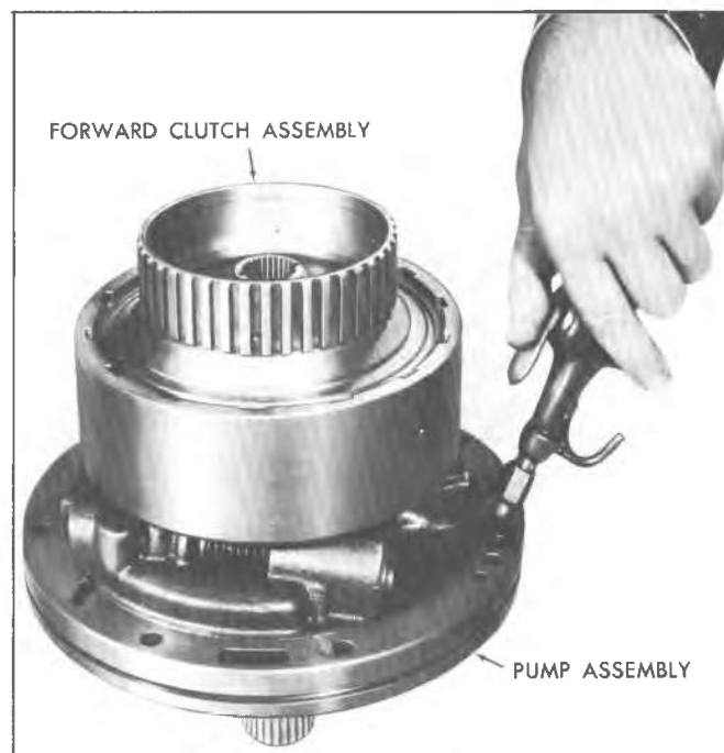
Fig. 7A-90C--Air Checking Forward Clutch Assembly
