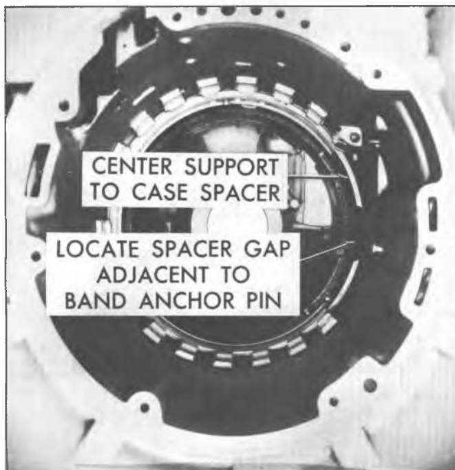
Fig. 7A-44C--Removing Center Support to Case Spacer
