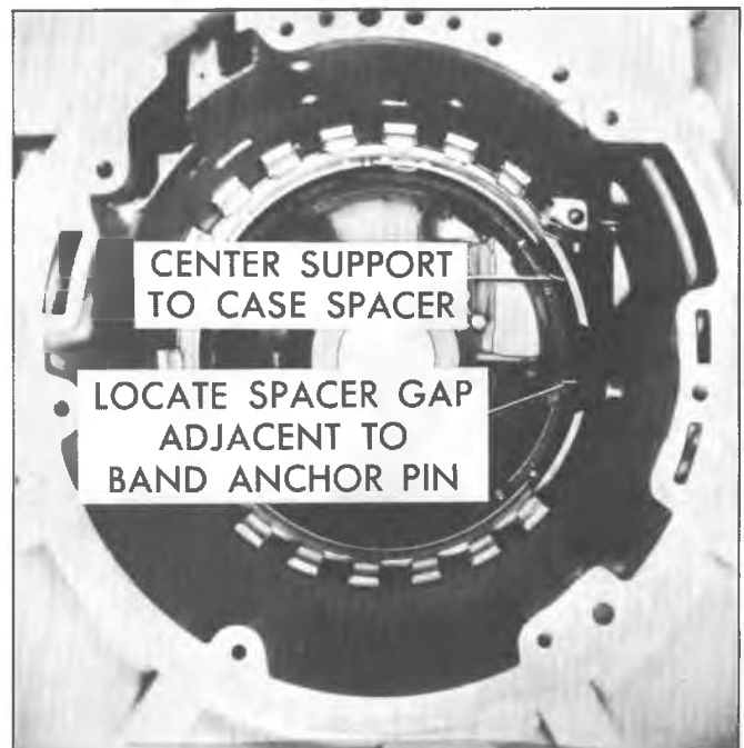
Fig. 7A-157C--Installing Center Support to Case Spacer
