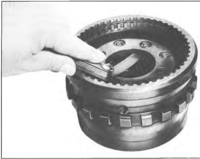
Fig. 7A-129C--Checking Output Carrier Pinion End Play
