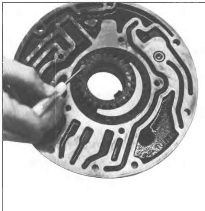
Fig. 7A-66B--Installing Pump Drive and Driven Gears
