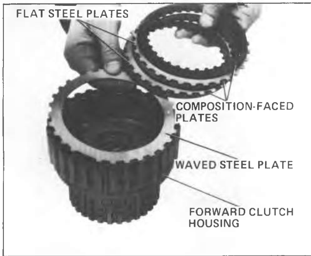
Fig. 7A-119A--Installing Clutch Plates Into Forward Clutch Housing
