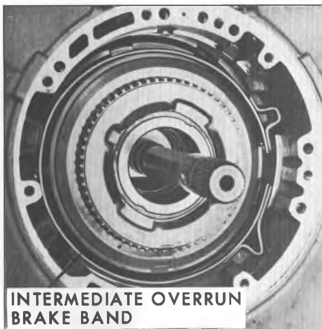
Fig. 7A-34B--Removing Intermediate Overrun Brake Band
