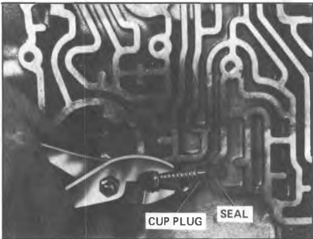
Fig. 7A-33A--Removing Cup Plug and Seal
