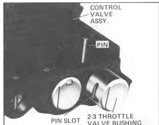
Fig. 7A-157A--Installing 2-3 Throttle Valve Bushing
