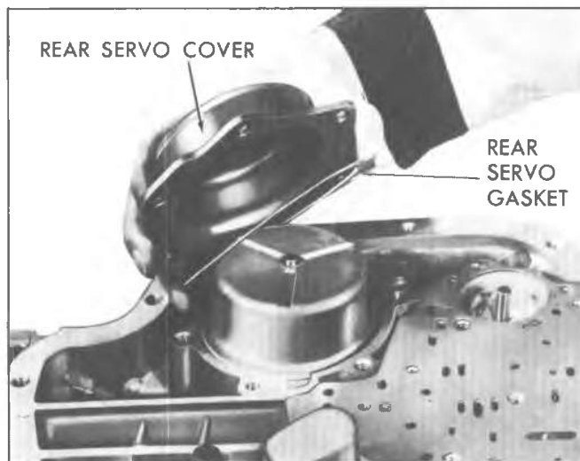
Fig. 7A-182C--Installing Rear Servo Cover and Gasket
