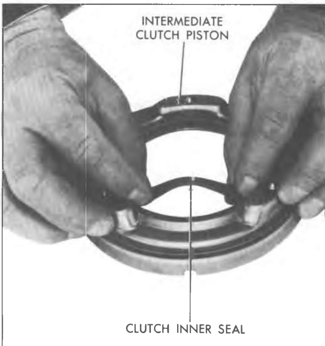
Fig. 7A-119C--Installing Intermediate Clutch Inner Seal
