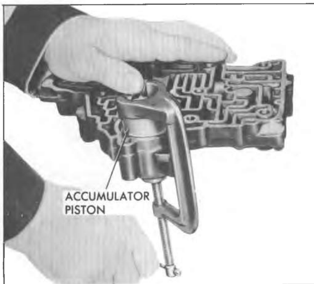
Fig. 7A-65C--Installing Compressor Tool to Front Accumulator Piston
