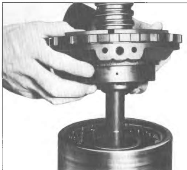
Fig. 7A-151C--Installing Center Support to Reaction Carrier
