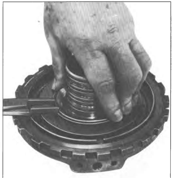
Fig. 7A-124C--Installing Intermediate Clutch Piston Snap Ring
