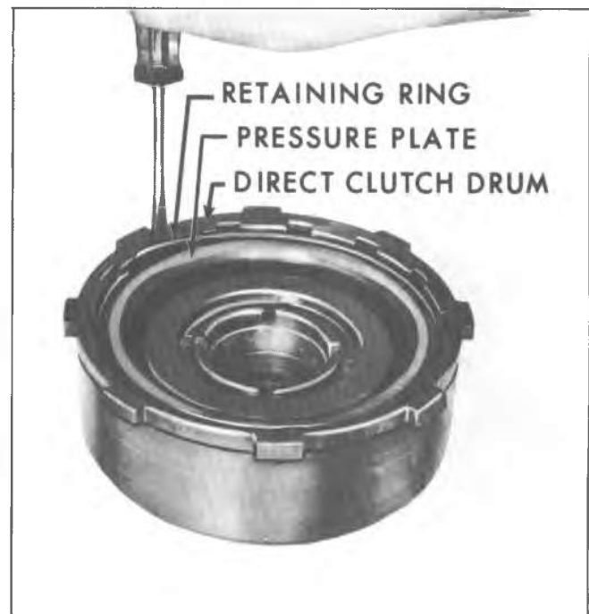
Fig. 7A-73B--Removing Direct Clutch Pressure Plate
