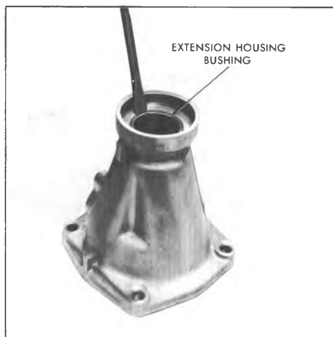
Fig. 7A-8B--Removing Extension Housing Bushing
