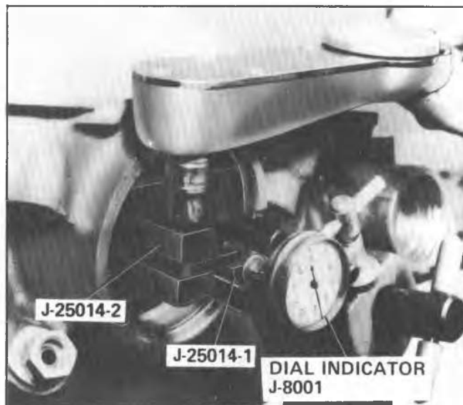
Fig. 7A-16A--Checking for Proper Intermediate Band Apply Pin
