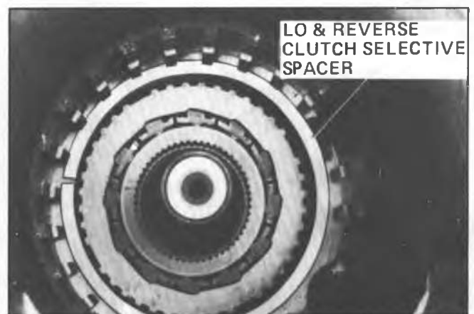
Fig. 7A-80A--Correct Location of Low and Reverse Clutch Selective Spacer
