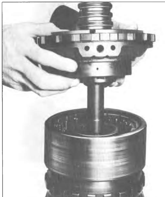
Fig. 7A-46C--Removing Center Support Assembly
