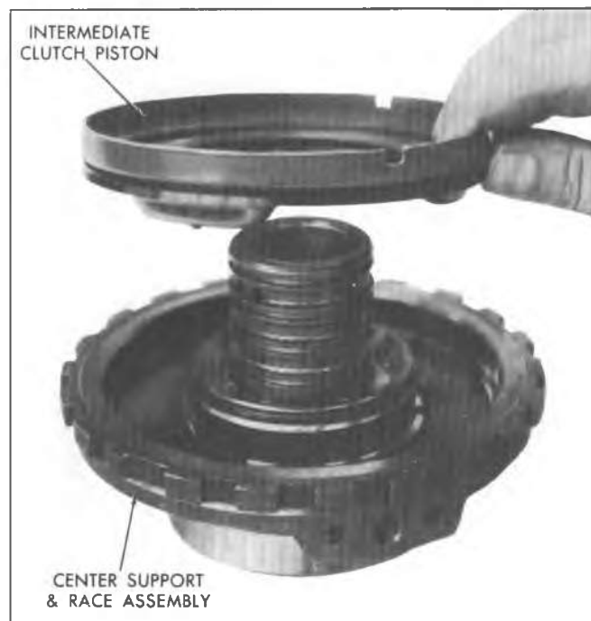
Fig. 7A-117C--Removing Intermediate Clutch Piston
