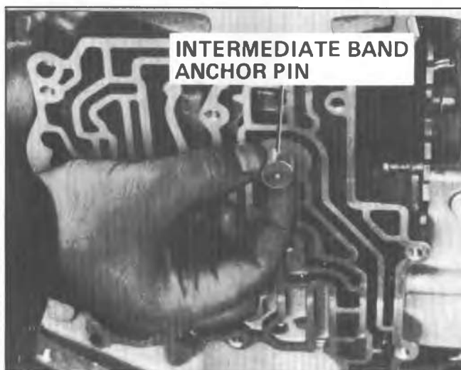
Fig. 7A-143A--Installing Intermediate Band Anchor Pin
