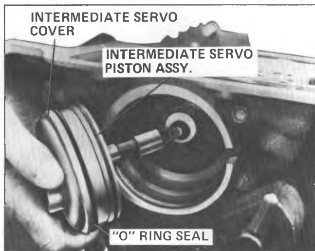
7A-150A--Installing Intermediate Servo Piston and Cover Assembly
