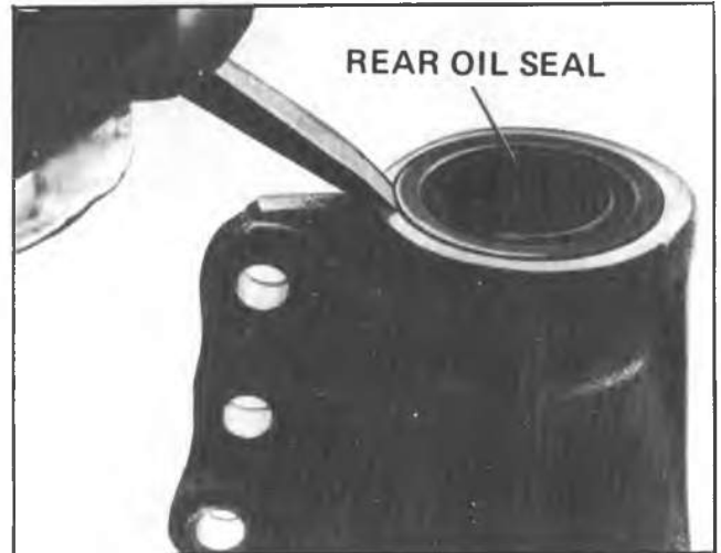
Fig. 7A-40A--Removing Rear Oil Seal
