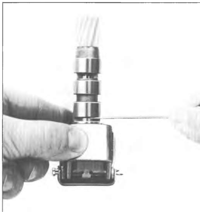
Fig. 7A-59C--Checking Valve Opening With Weight Inward
