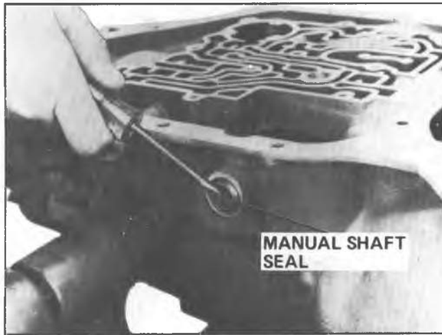
Fig. 7A-44A--Removing Manual Shaft Seal From Case
