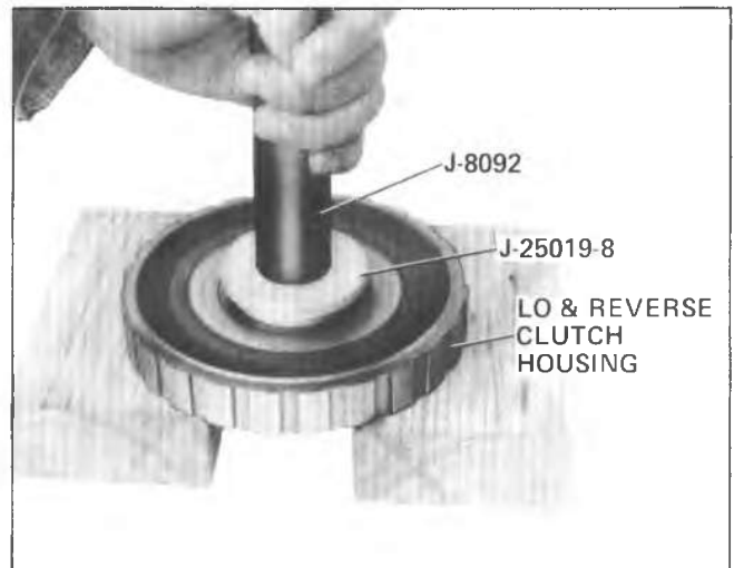
Fig. 7A-183A--Installing Lo and Reverse Clutch Housing Bushing
