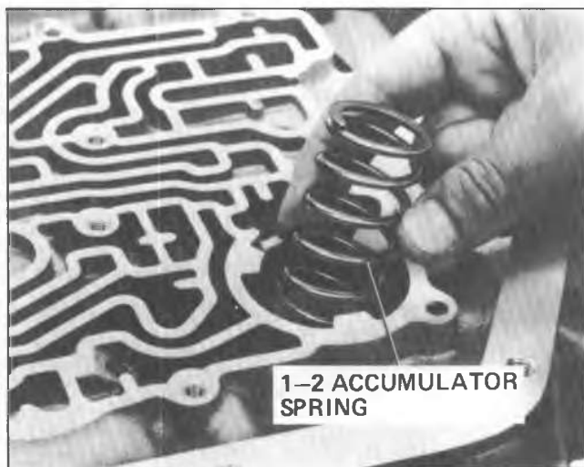
Fig. 7A-158A--Installing 1-2 Accumulator Spring
