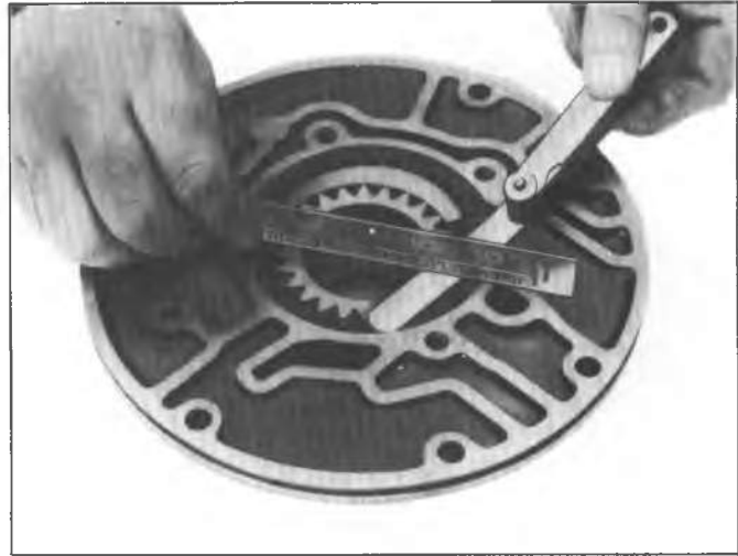
Fig. 7A-134A--Checking Pump Body-to-Gear End Clearance
