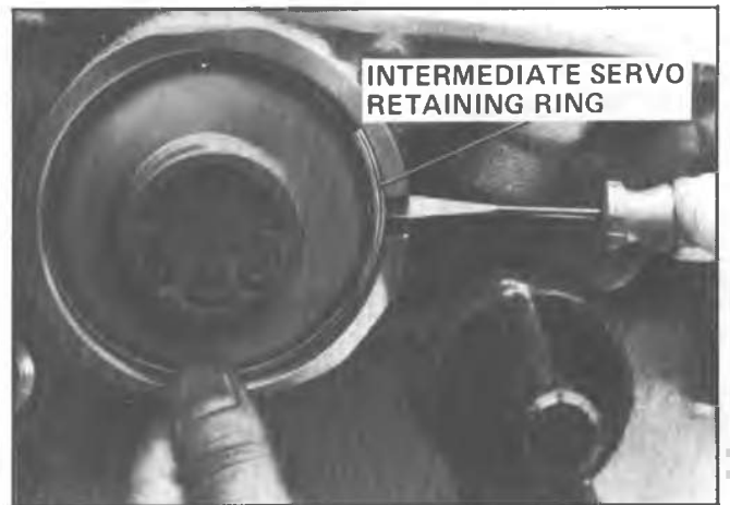
Fig. 7A-11A--Removing Intermediate Servo Retaining Ring
