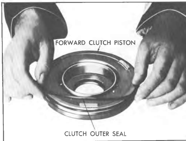
Fig. 7A-84C--Removing Forward Clutch Piston Outer Seal
