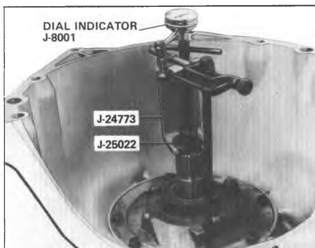
Fig. 7A-139A--Checking Front Unit End Play
