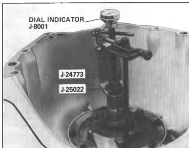
Fig. 7A-19A--Checking Front Unit End Play
