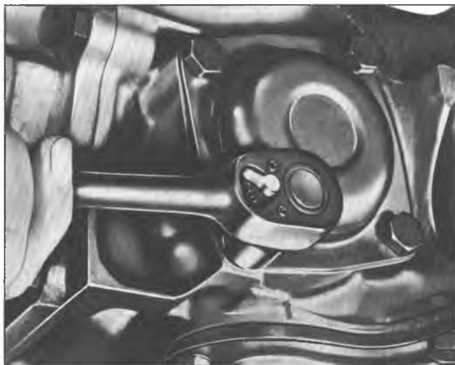
Fig. 7A-5C--Removing Governor Cover Attaching Screws
