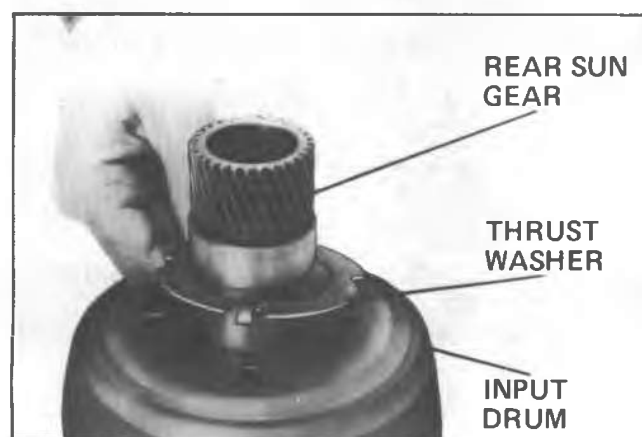
Fig. 7A-86A--Installing Thrust Washer
