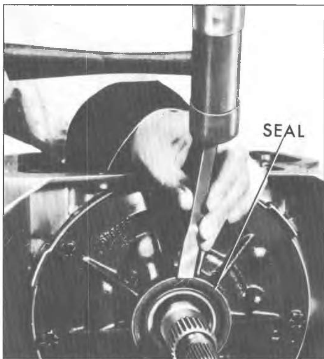
Fig. 7A-31C--Removing Front Seal
