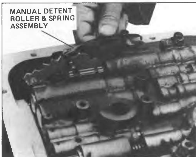
Fig. 7A-163A--Installing Manual Detent Roller and Spring Assembly
