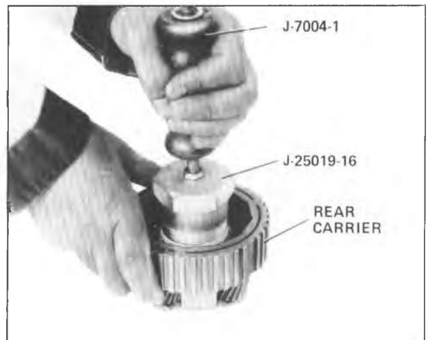
Fig. 7A-184A--Removing Rear Carrier Bushing
