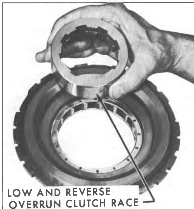
Fig. 7A-94B--Removing Overrun Clutch Inner Race
