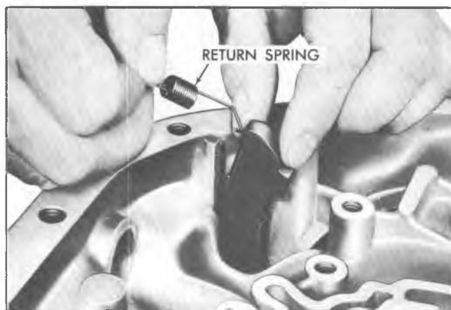
Fig. 7A-24C--Removing Parking Pawl Return Spring
