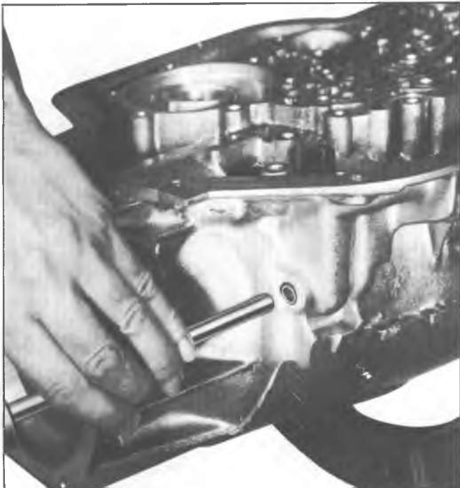
Fig. 7A-154C--Installing Parking Pawl Shaft Cup Plug
