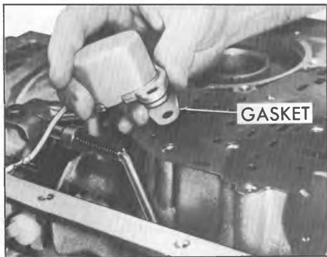
Fig. 7A-18C--Removing Detent Solenoid and Gasket
