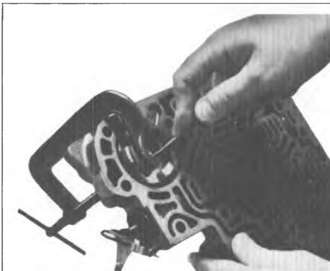
Fig. 7A-55B--Removing Direct Clutch Accumulator Piston Retaining "E" Ring
