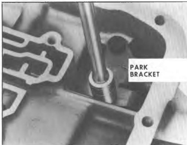
Fig. 7A-45A--Removing Parking Pawl Bracket Bolt
