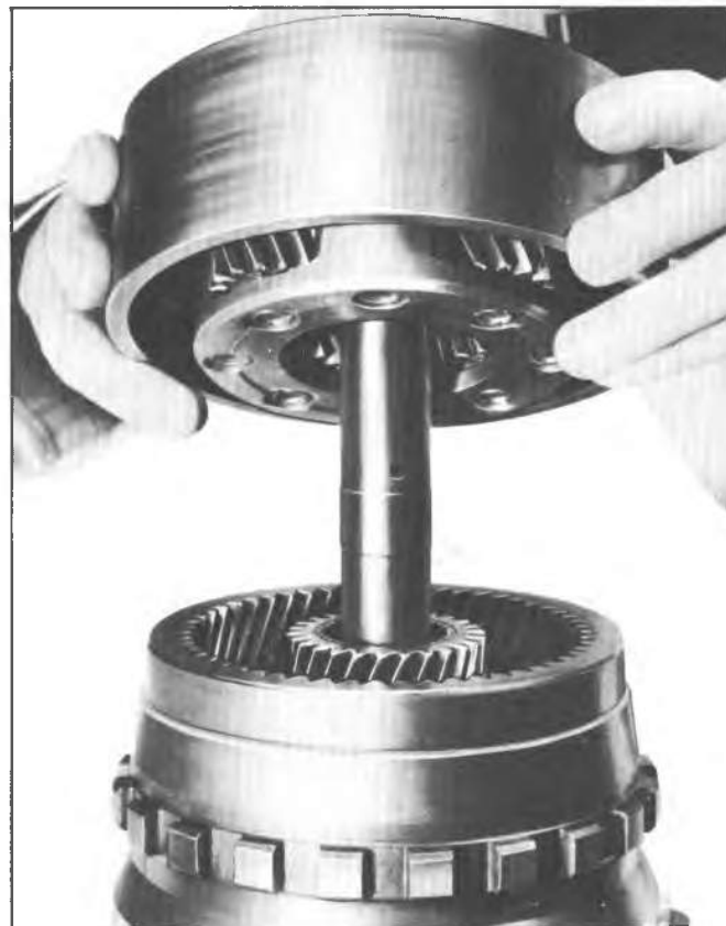
Fig. 7A-147C--Installing Reaction Carrier
