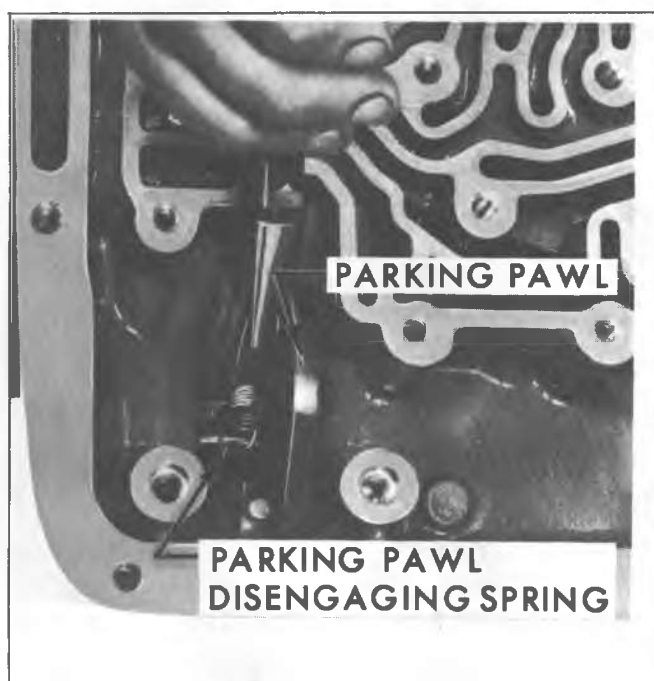
Fig. 7A-26B--Removing Parking Pawl Disengaging Spring
