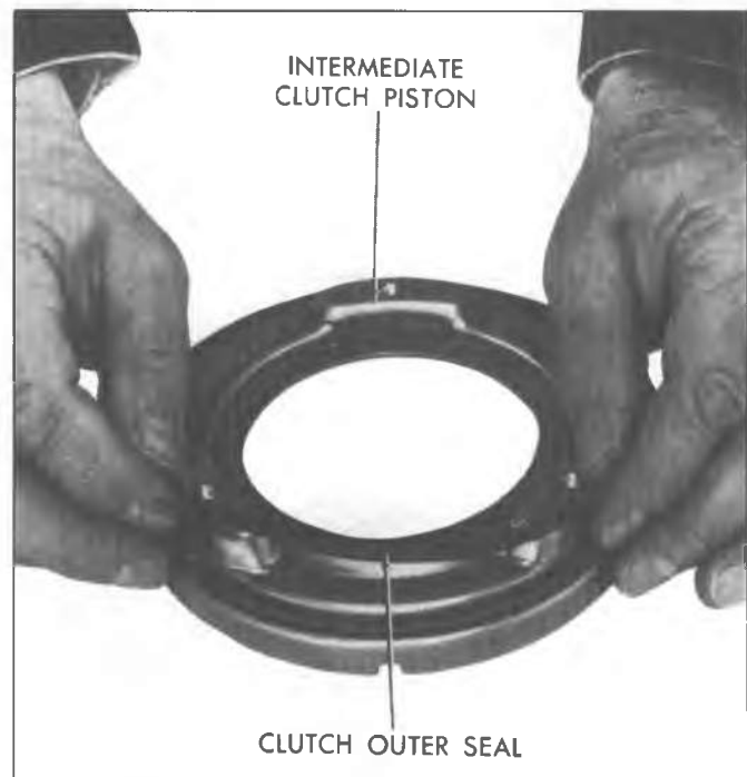
Fig. 7A-120C--Installing Intermediate Clutch Outer Seal
