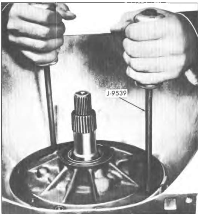
Fig. 7A-32C--Removing Pump Assembly
