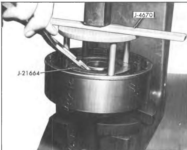
Fig. 7A-94C--Removing or Installing Direct Clutch Snap Ring
