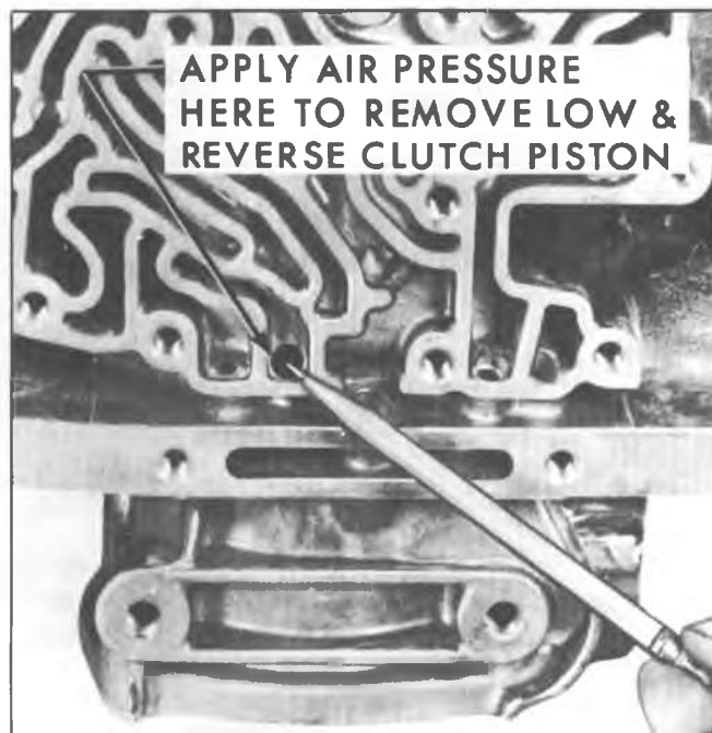
Fig. 7A-50B--Removing Low and Reverse Clutch Piston
