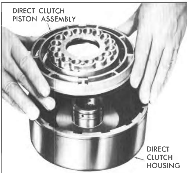
Fig. 7A-95C--Removing Direct Clutch Piston Assembly
