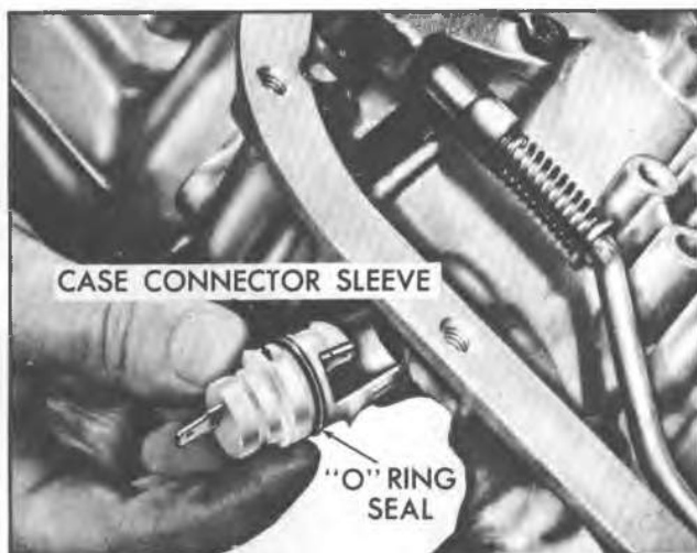
Fig. 7A-178C--Installing Electrical Connector and "O" Ring Seal
