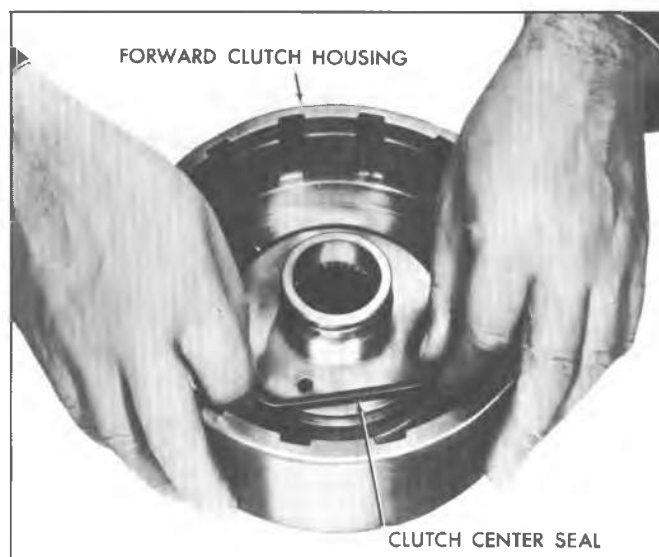
Fig. 7A-85C--Removing Forward Clutch Center Seal
