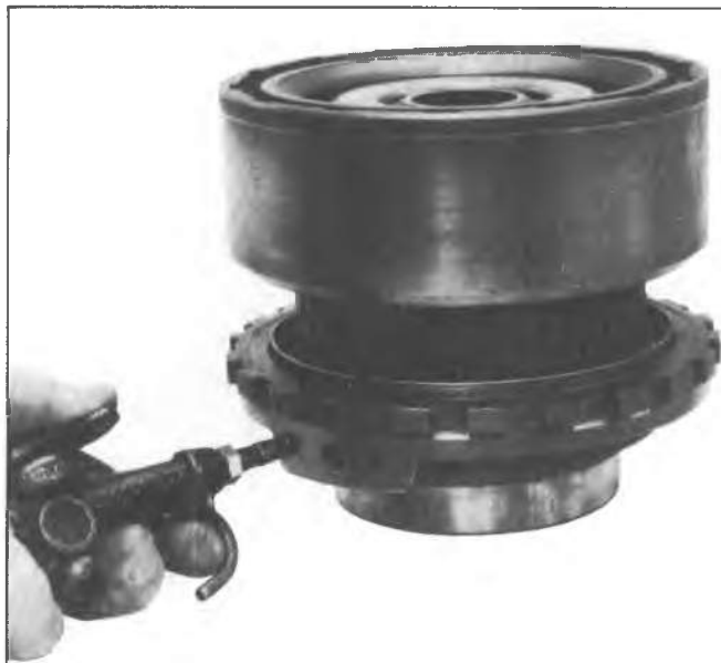
Fig. 7A-111C--Air Checking Direct Clutch Assembly
