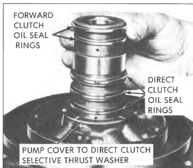
Fig. 7A-61B--Pump Hub Oil Seal Rings
