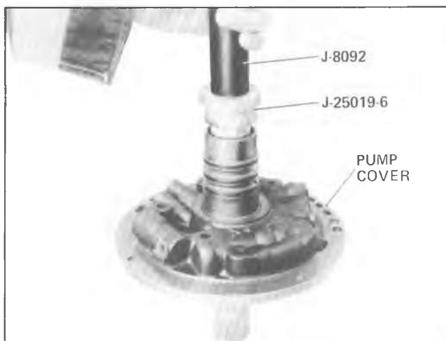
Fig. 7A-171A--Installing Pump Cover Bushing - Rear
