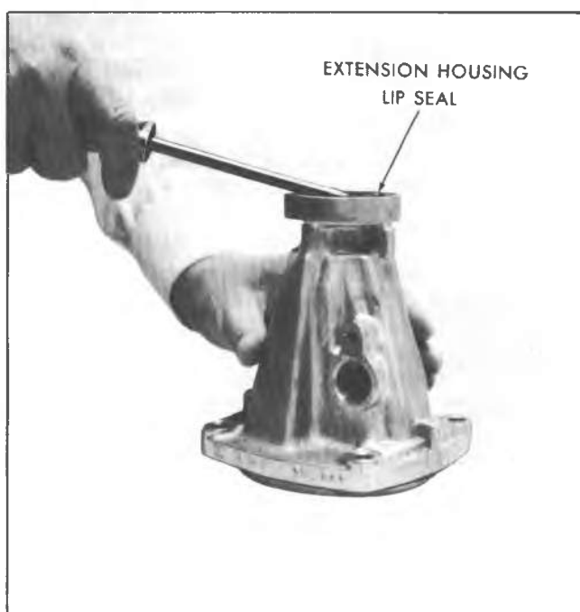
Fig. 7A-7B--Removing Extension Housing Lip Seal
