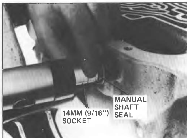
Fig. 7A-53A--Installing Manual Shaft Seal Into Case
