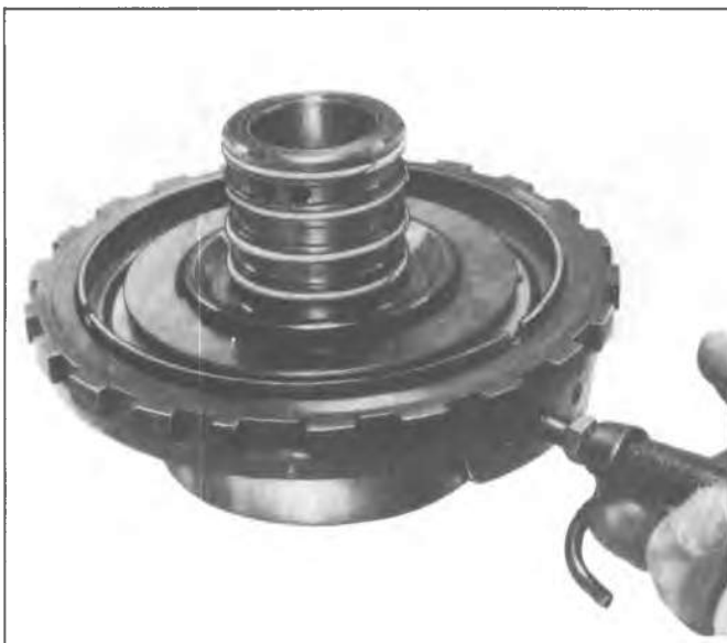
Fig. 7A-126C--Air Checking Intermediate Clutch Piston
