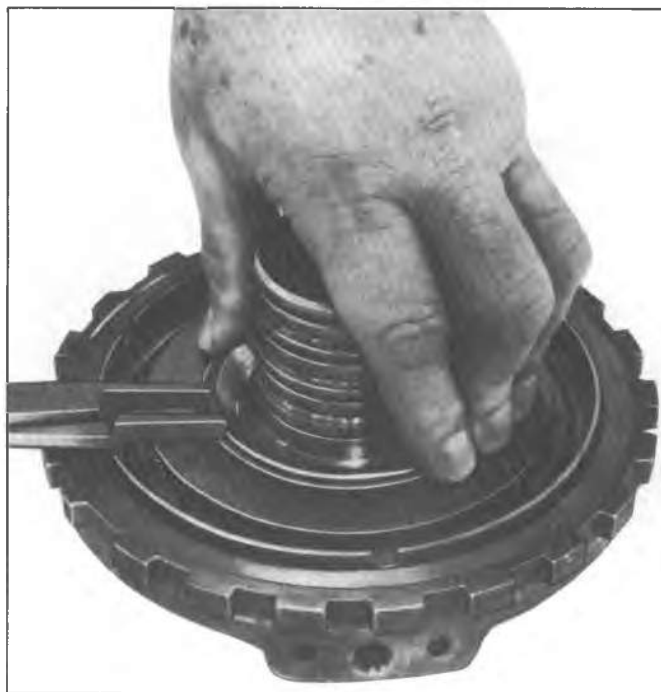
Fig. 7A-113C--Removing Intermediate Clutch Piston Snap Ring
