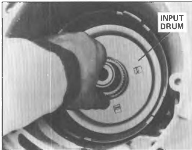
Fig. 7A-32A--Removing Input Drum and Rear Sun Gear
