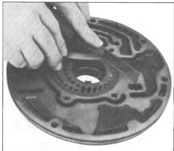
Fig. 7A-74C--Checking Pump Body Face to Gear Face Clearance
