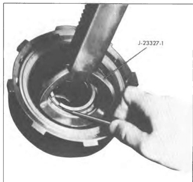
Fig. 7A-75B--Compressing Direct Clutch Spring Seat
