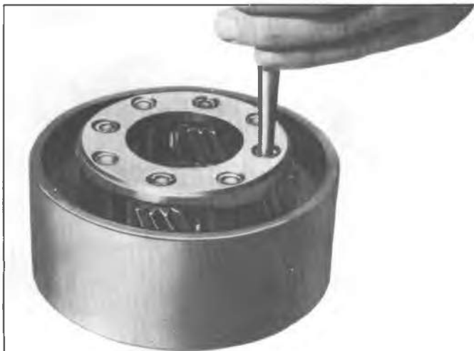
Fig. 7A-130C--Removing Planet Pinion Pin
