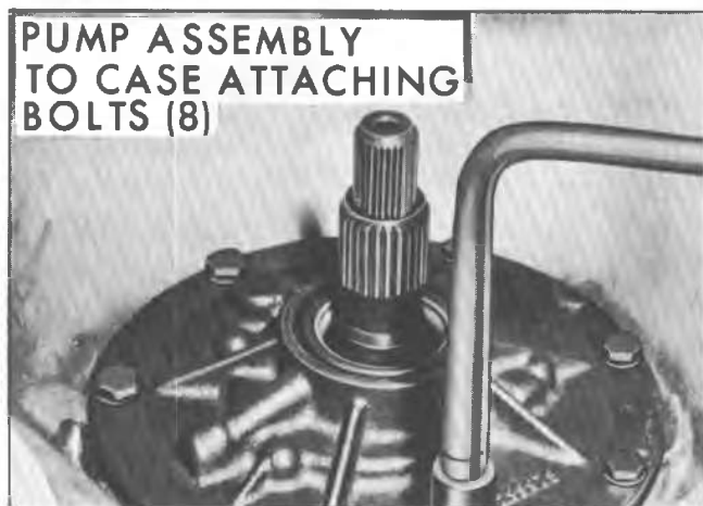
Fig. 7A-29B--Removing Pump Attaching Bolts
