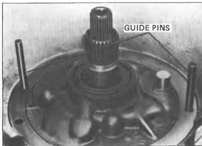
Fig. 7A-138A--Installing Pump Assembly
