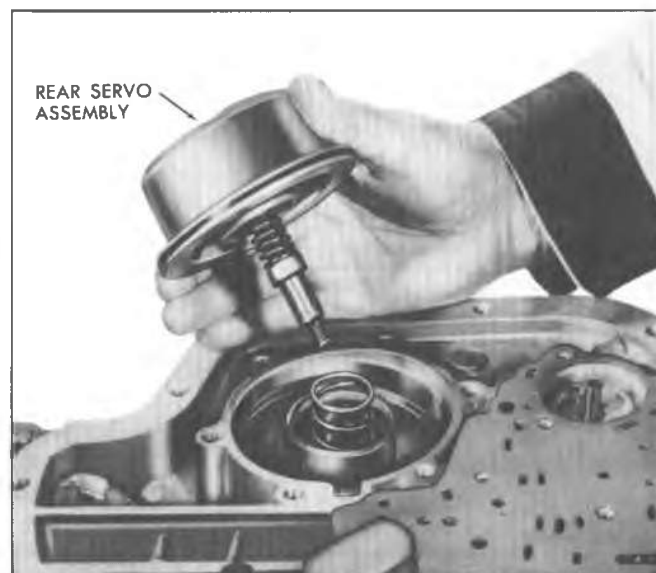
Fig. 7A-14C--Removing Rear Servo Assembly
