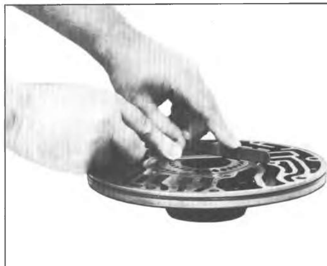
Fig. 7A-63B--Checking Pump Body to Gear Face Clearance
