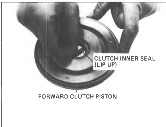
Fig. 7A-115A--Removing or Installing Inner Piston Seal
