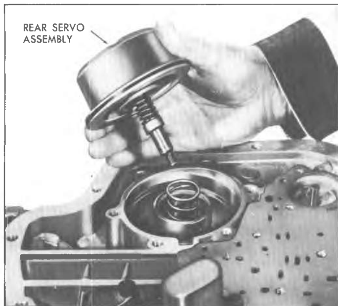
Fig. 7A-181C--Installing Rear Servo Assembly
