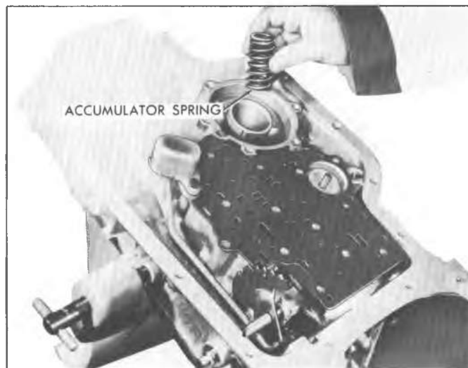
Fig. 7A-180C--Installing Rear Accumulator Spring
