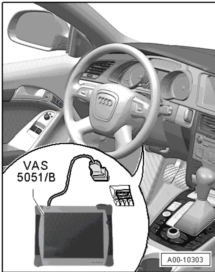
Fig. 16: Connecting Diagnostic Cable VAS 5051/5A To Diagnostic Connector Courtesy of AUDI OF AMERICA, LLC
