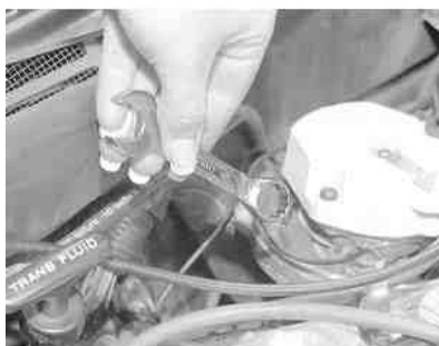
Fig. 5: The easiest way to loosen the distributor hold-down bolt is with a stubby wrench
