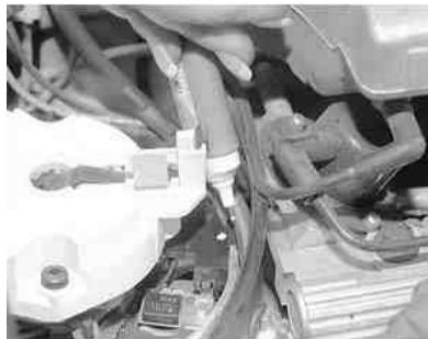
Fig. 3: Use a paint marker to matchmark the position of the rotor to the distributor housing
