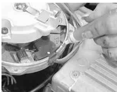
Fig. 7: Pull the distributor up until the rotor just stops turning, then mark the rotor position again
