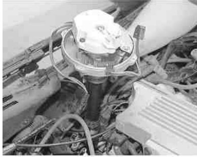
Fig. 9: Place a rag or shop towel in the distributor mounting hole to prevent debris from falling into the engine
