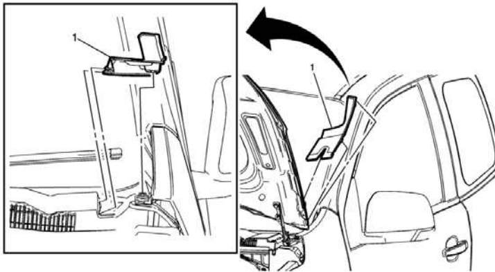
Air Inlet Grille Panel Extension Replacement
