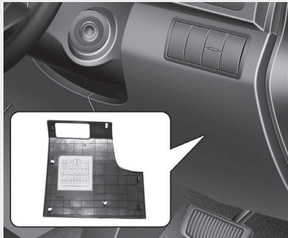
Inner fuse panel
