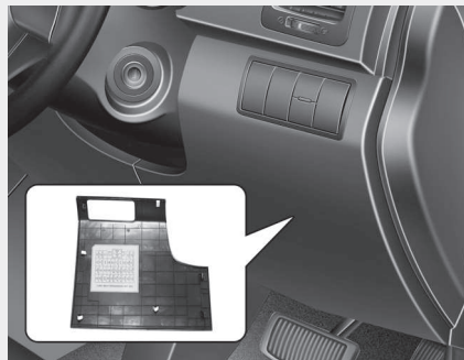
Inner fuse panel
