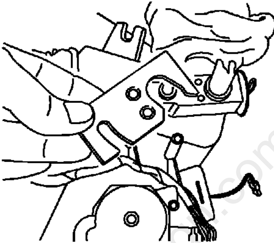
Fig. 51: View Of TXV Line Bracket Courtesy of GENERAL MOTORS COMPANY
