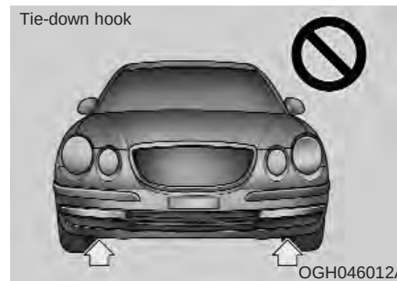
Tie-down hook (for flatbed towing)
