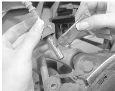
Fig. 22: Apply some silicone grease to the guide pin before reinstalling it
