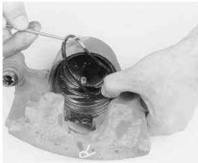
Fig. 6: Use extreme caution when removing the piston seal; DO NOT scratch the caliper bore
