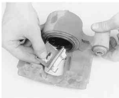
Fig. 3: On some vehicles, you must remove the anti-rattle clip
