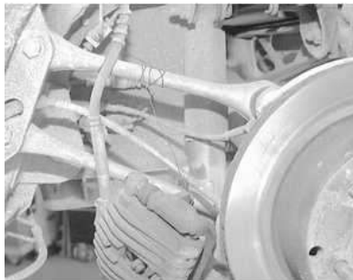
Fig. 21: Hang the caliper from the suspension with a piece of mechanic's wire. NEVER let the caliper hang by the brake line!
