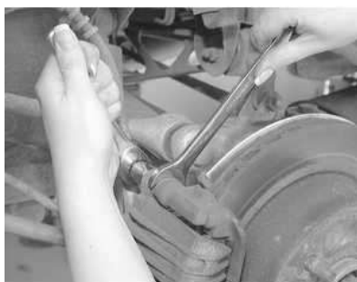
Fig. 11: Hold the guide pin stationary with one wrench, then loosen the top caliper self-locking bolt
