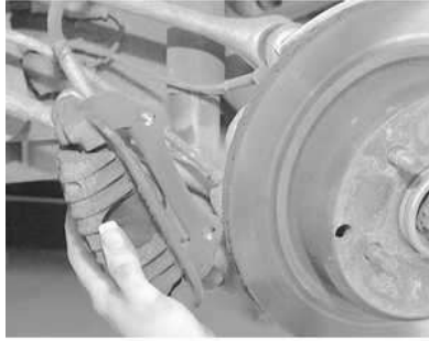
Fig. 21: Hang the caliper from the suspension with a piece of mechanic's wire. NEVER let the caliper hang by the brake line!
