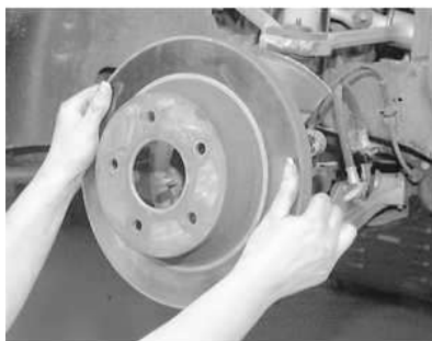
Fig. 2: Install the rotor by positioning it over the lug studs, and pushing it into place — front rotor shown
