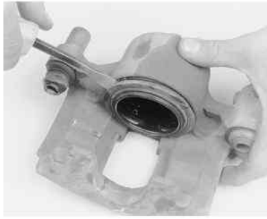
Fig. 4: Remove the bolt, then rotate the caliper down for access to the pads
