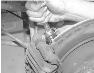
Fig. 18: Loosen the upper caliper bracket mounting bolt . . .
