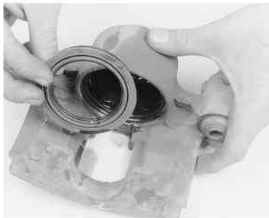
Fig. 5: ... then remove the boot from the caliper housing, taking care not to score or damage the bore
