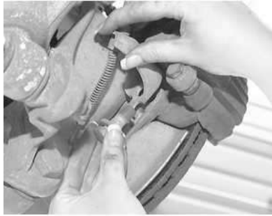
Fig. 17: Remove the lower bolt and position the parking brake cable and bracket aside
