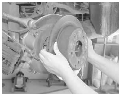
Fig. 1: Remove the rotor by lifting it straight off the lug studs — rear rotor shown
