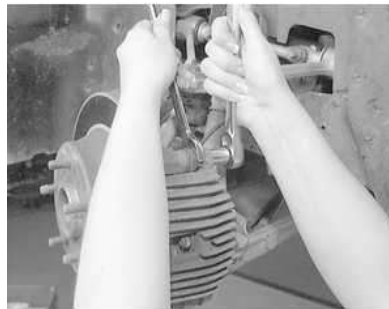
Fig. 2: While holding the guide pin bolt stationary with a wrench, loosen the top caliper self-locking bolt
