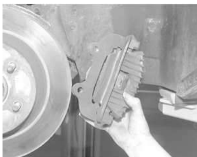
Fig. 4: Then, you can remove the entire caliper and brake assembly from the vehicle
