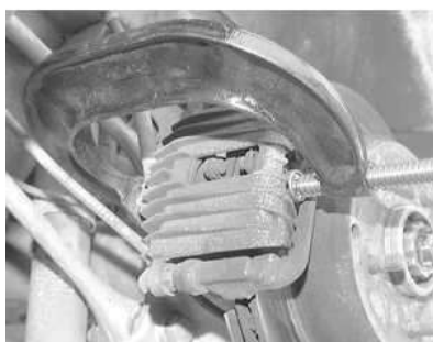
Fig. 10: Position a C-clamp so one end rests on the inlet fitting bolt head and the other end against the outboard shoe. Tighten until the piston is bottomed out in the bore
