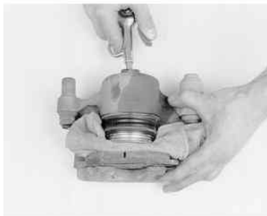
Fig. 1: For some types of calipers, use compressed air to drive the piston out of the caliper, but make sure to keep your fingers clear
