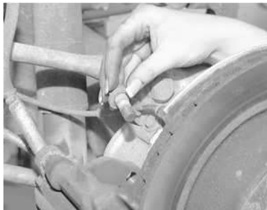
Fig. 19: . . . then pull the bolt out of the rear of the bracket
