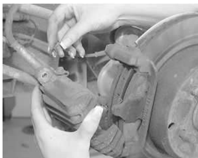
Fig. 8: Remove the bolt, then rotate the caliper down for access to the pads
