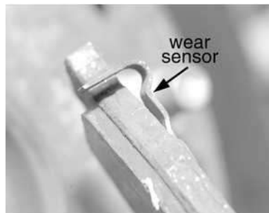
Fig. 10: The inboard rear brake pad usually has a wear sensor to let you know your brakes are getting low
