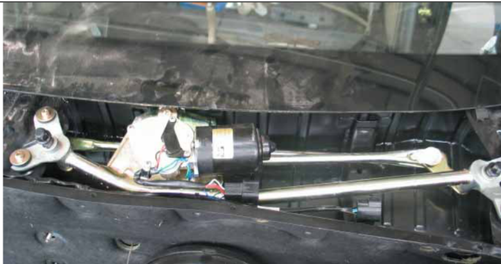
Installation of the wiper abutment
