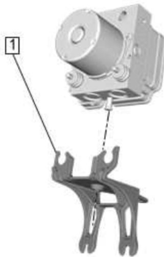
Fig. 30: Brake Pressure Modulator Valve Bracket Courtesy of GENERAL MOTORS COMPANY
