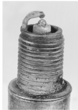
Fig. 7: Inspect the spark plug to determine engine running conditions
