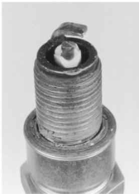
Fig. 7: Inspect the spark plug to determine engine running conditions
