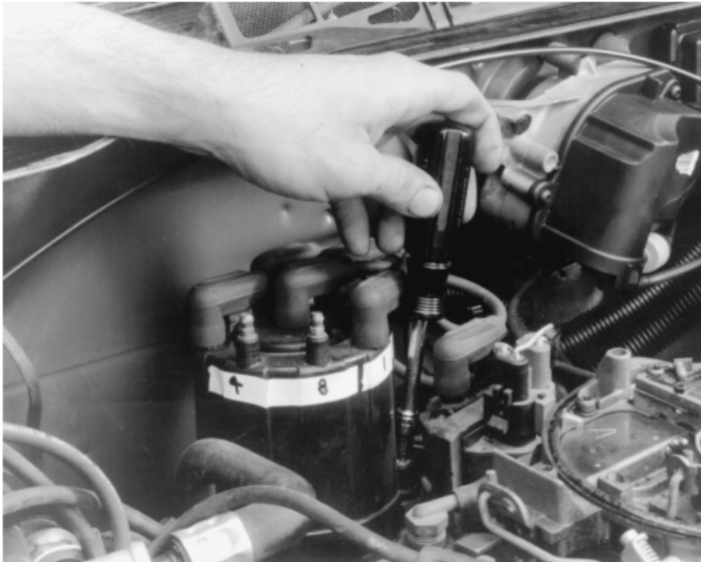
Fig. 5: Release the retainers on the distributor cap by turning them counterclockwise
