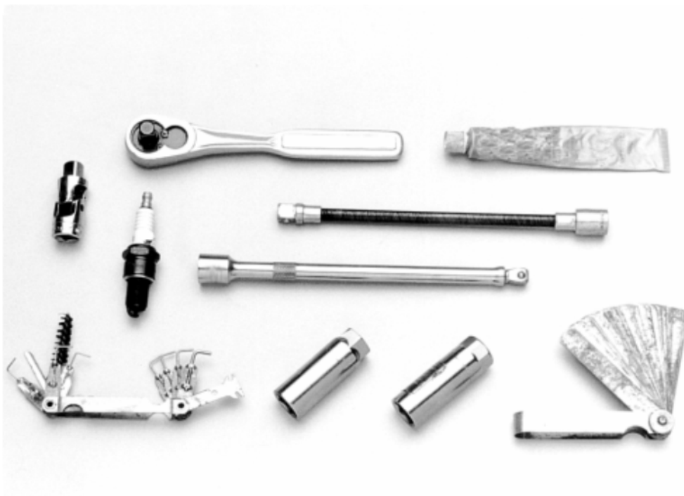
Fig. 2: A variety of tools and gauges are needed for spark plug service
