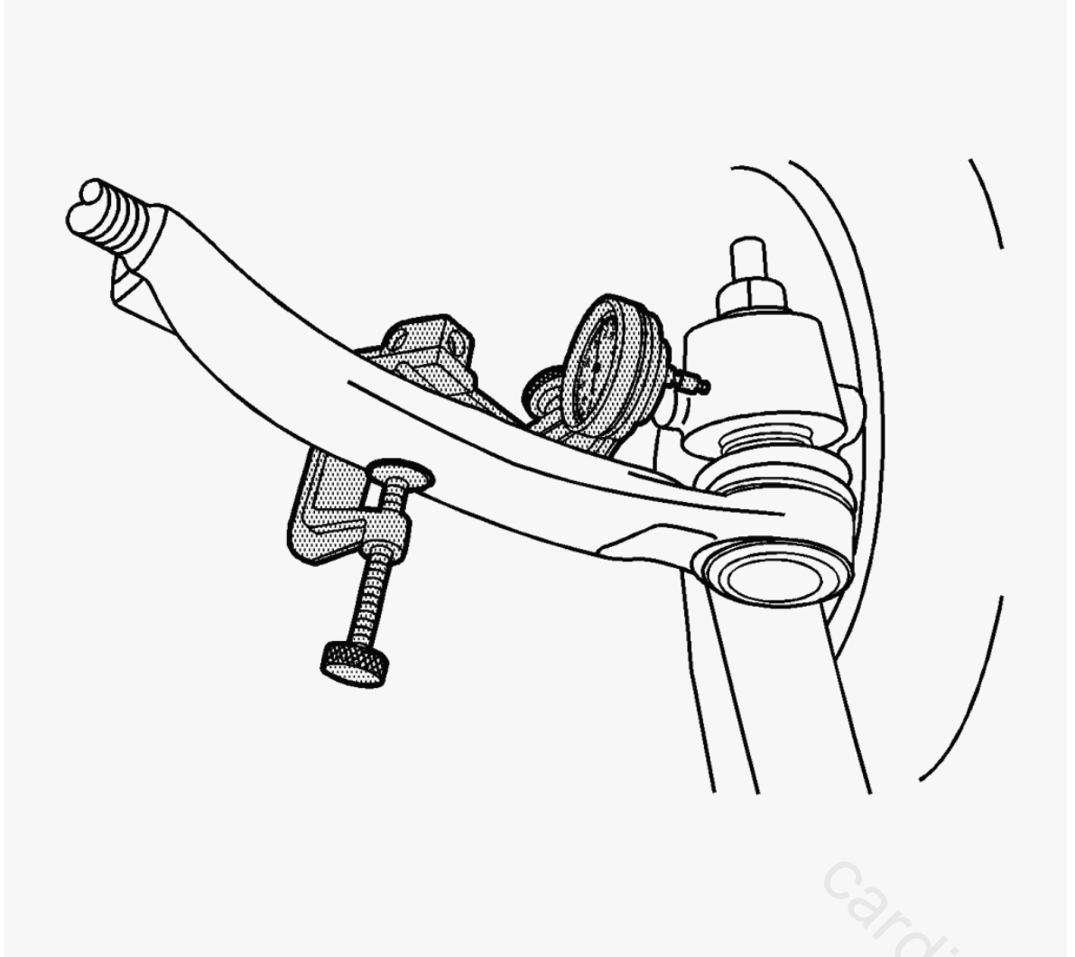
Fig. 12: Measuring Outer Tie Rod Lash
