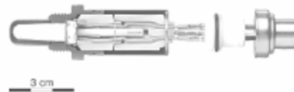
Interior structure of oxygen sensor
