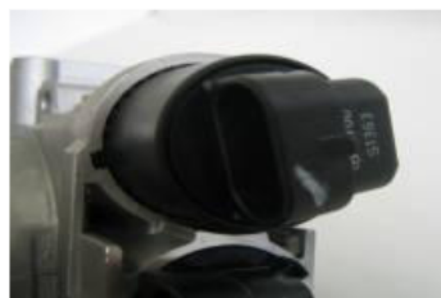
Idle actuator with step motor
