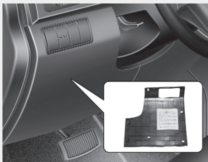
Inner fuse panel
