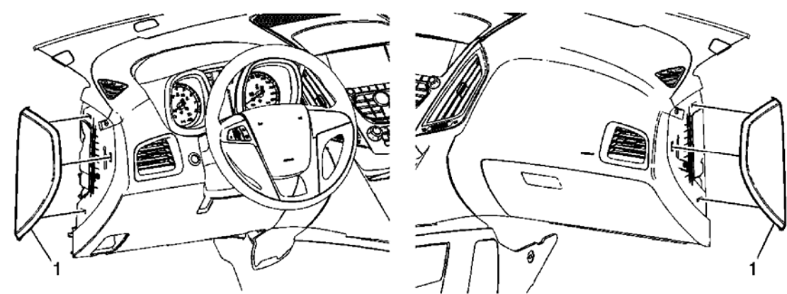
Fig. 9: Instrument Panel Side Trim Panel (Equinox) Courtesy of GENERAL MOTORS CORP.
