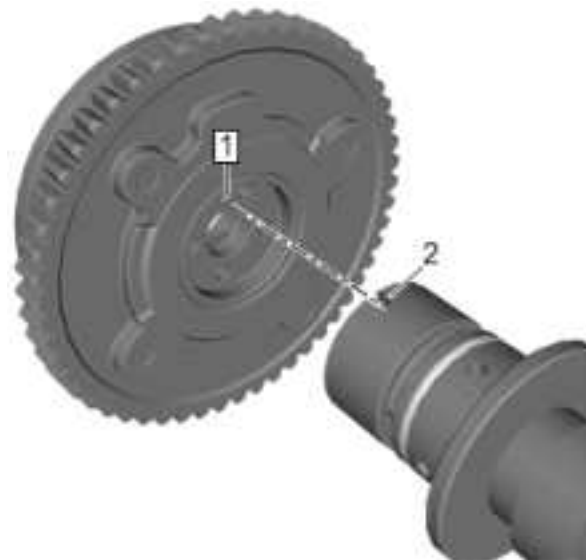
Fig. 69: Dowel Pin And Camshaft Slot Courtesy of GENERAL MOTORS COMPANY
