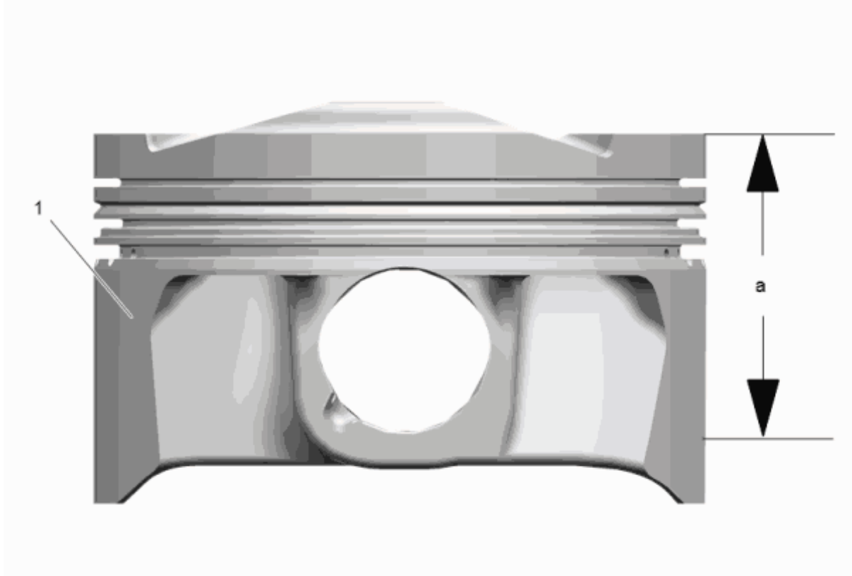
Fig. 418: Measuring Piston Width
