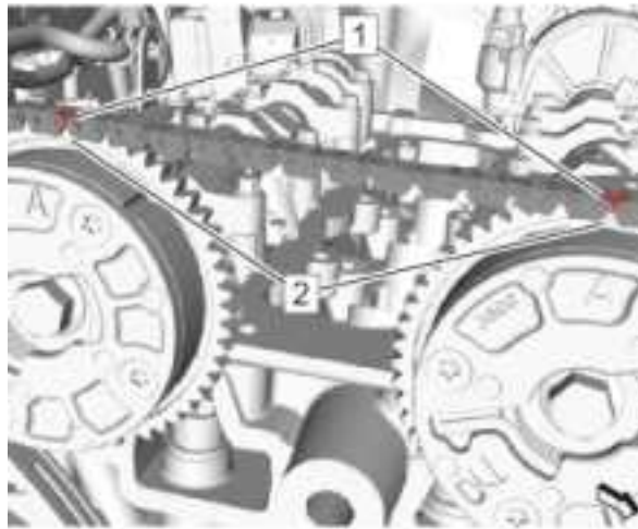
Fig. 72: Camshaft Position Actuator Marks And Timing Chain Marks Courtesy of GENERAL MOTORS COMPANY
