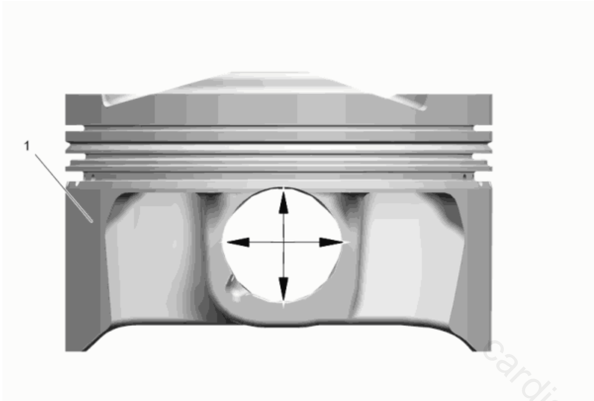
Fig. 420: Measuring Piston Pin Bore Courtesy of GENERAL MOTORS COMPANY
