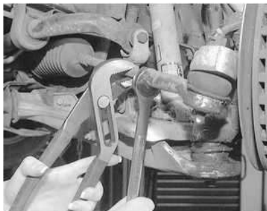
Fig. 2: Use pliers to hold the inner tie rod end, then loosen the jam nut
