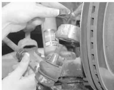
Fig. 7: Unfasten the slotted nut, then remove the tie rod end from the steering knuckle
