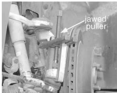
Fig. 5: Install a suitable jawed puller to separate the tie rod end from the steering knuckle
