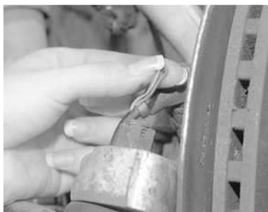
Fig. 3: Remove the cotter pin from the slotted nut
