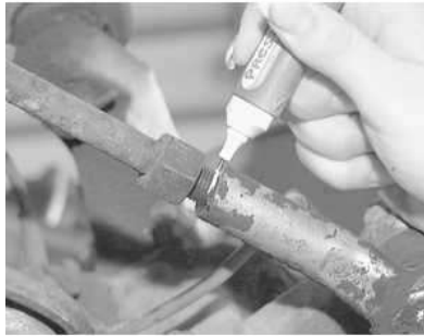
Fig. 1: Make sure you matchmark the installed position of the tie rod end for proper alignment during installation
