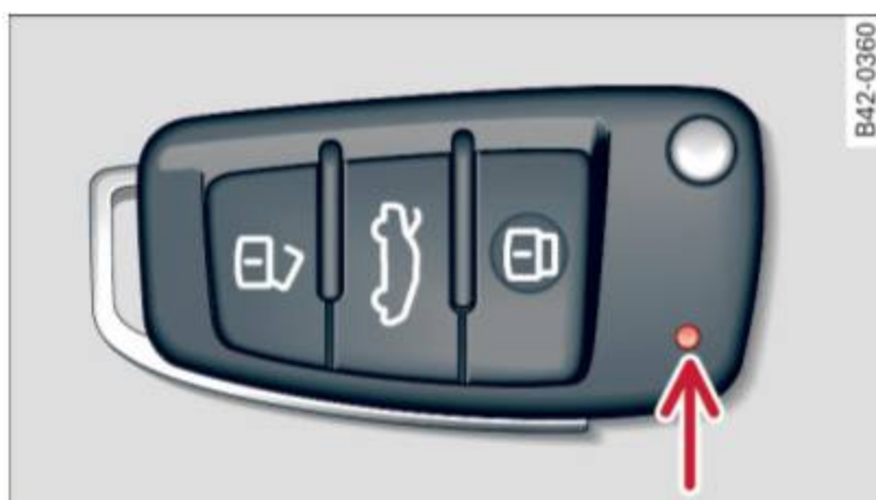
Fig. 21 Remote master key: Indicator light
