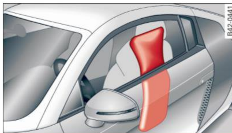
Fig. 99 Inflated side airbags on left side of vehicle
