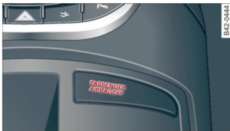
Fig. 95 Section from the instrument panel: PASSENGER AIR BAG OFF light
