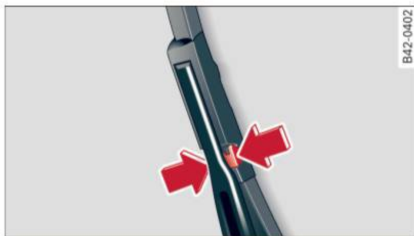
Fig. 41 Unlatching wiper blades
