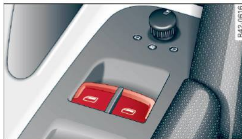
Fig. 31 Driver's door: power window switches
