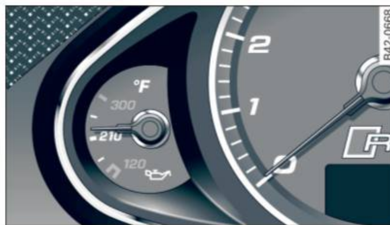
Fig. 114 Instrument cluster: Engine oil temperature display
