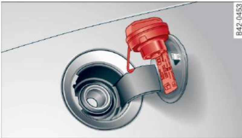
Fig. 108 Fuel cap hooked on the opened fuel filler flap
