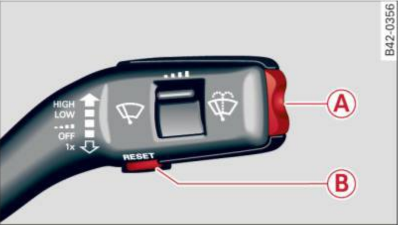
Fig. 12 Wiper lever: Controls for the menu display
