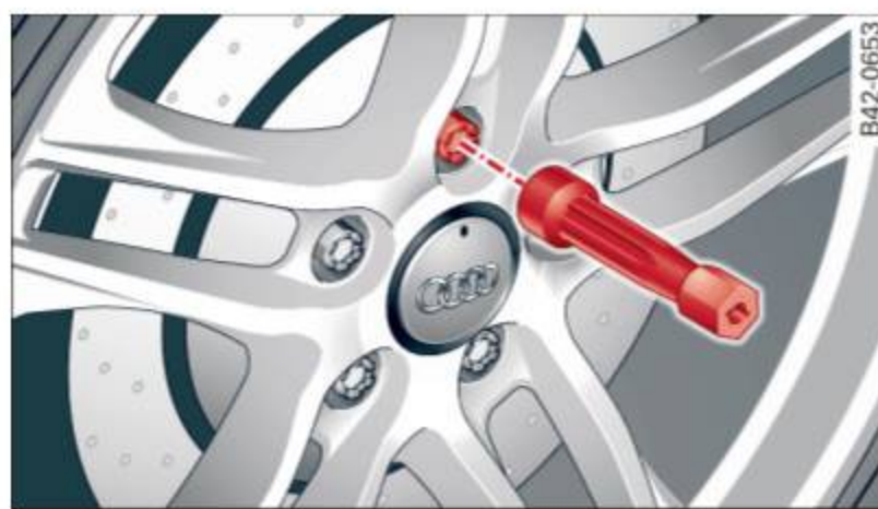
Fig. 136 Wheel change: using the screwdriver handle (with the blade removed) to turn the bolts
