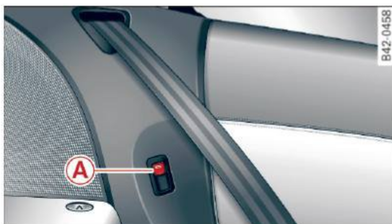
Fig. 110 Driver's side: releasing the engine compartment lid
