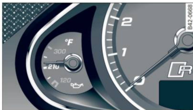
Fig. 116 Instrument cluster: Engine oil temperature display
