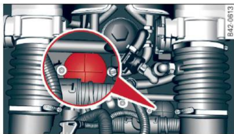
Fig. 65 Engine compartment: emergency release
