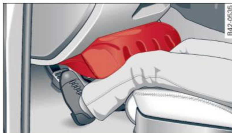
Fig. 97 Inflated airbags protecting in a frontal collision
