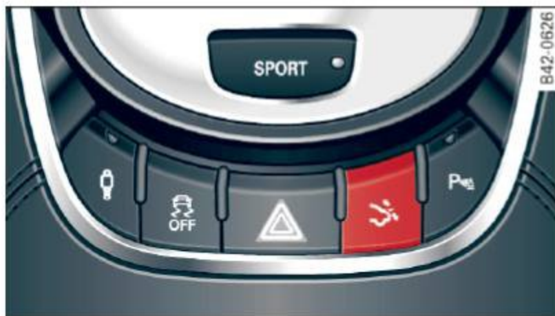
Fig. 106 Switch for rear spoiler
