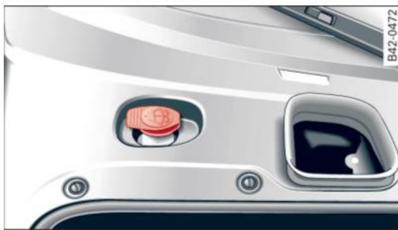
Fig. 123 Luggage compartment: Windshield washer fluid reservoir
