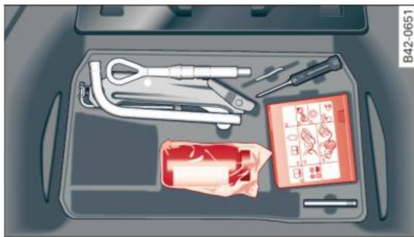
Fig. 130 Tire Mobility System under luggage compartment floor
