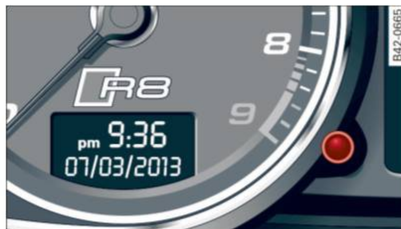
Fig. 56 Section of instrument cluster: Set/Check button
