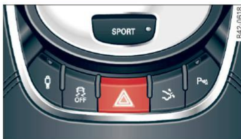
Fig. 34 Center console: emergency flasher switch
