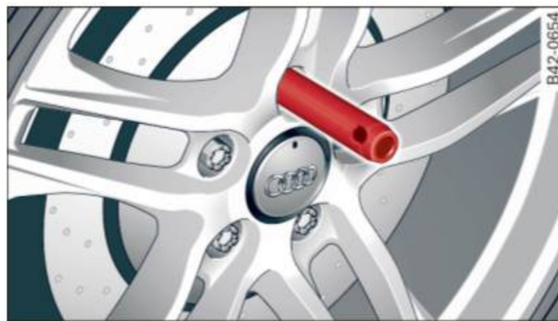
Fig. 137 Wheel change: alignment pin inside the top hole
