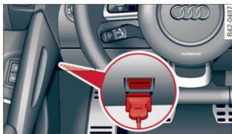
Fig. 19 Location of Data Link Connector (DLC)
