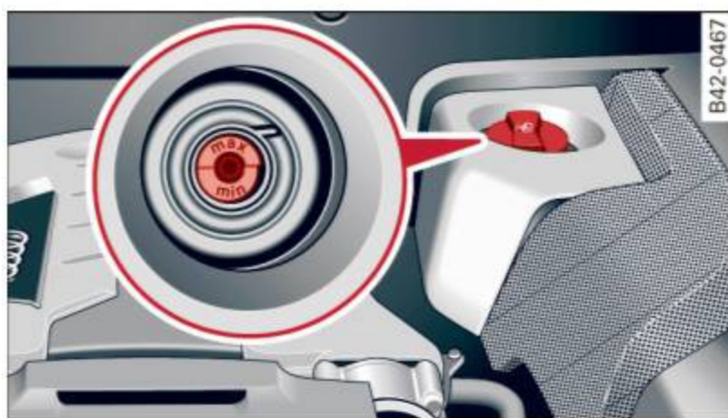
Fig. 120 Engine compartment: coolant expansion tank
