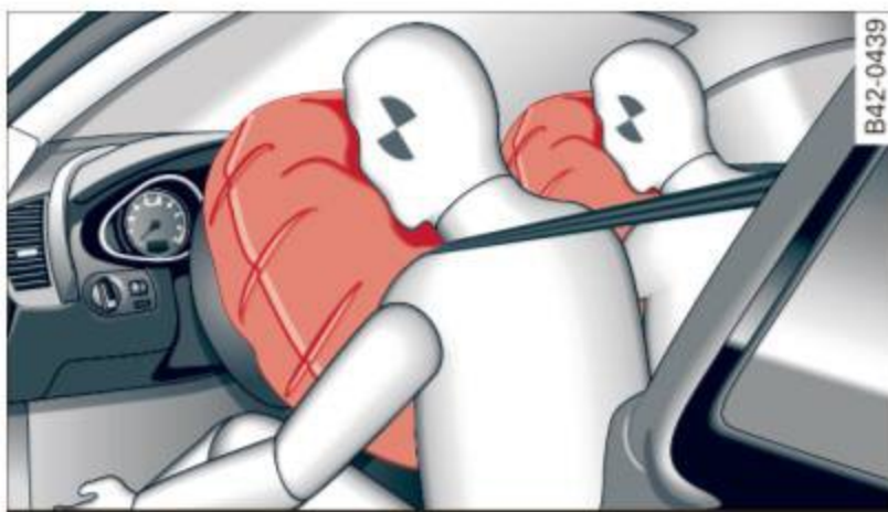
Fig. 94 Inflated front airbags
