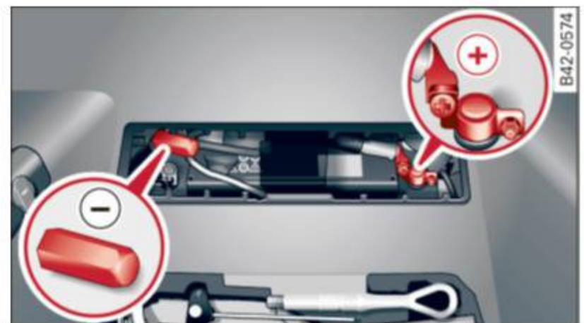
Fig. 122 Luggage compartment: connectors for a charger and jump start cables
