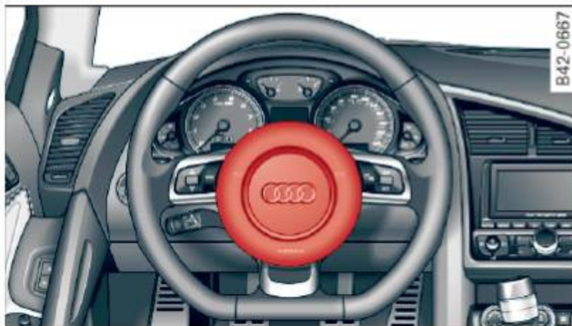
Fig. 92 Location of driver airbag: in steering wheel
