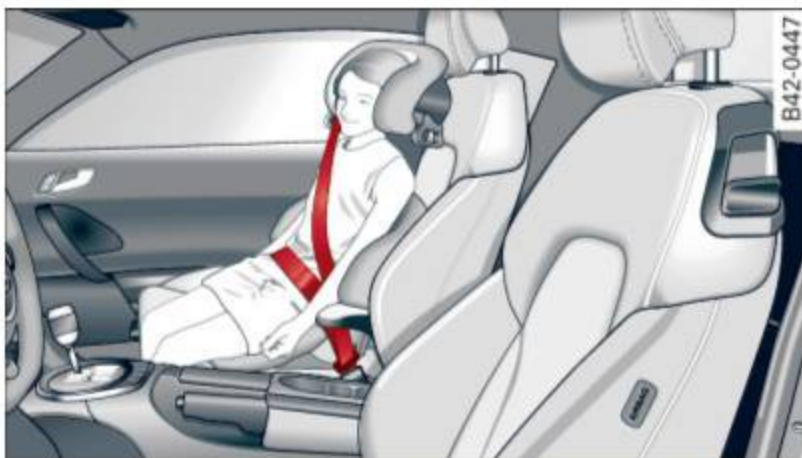
Fig. 102 Passenger seat: child properly restrained in a booster seat
