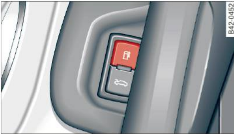
Fig. 107 Driver's door: Unlocking fuel filler flap
