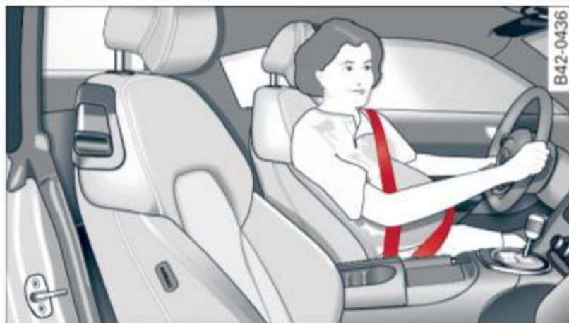
Fig. 90 Safety belt position during pregnancy
