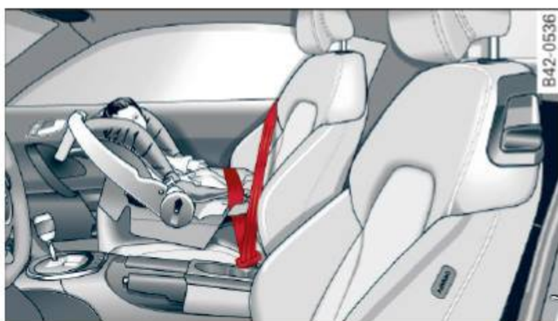
Fig. 100 Rearward-facing infant seat, properly installed on the passenger seat
