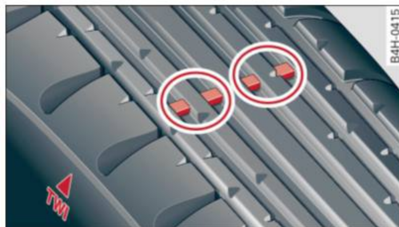
Fig. 126 Tire tread: tread wear indicators (TWI)
