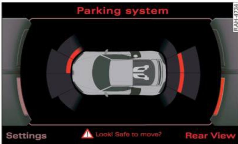
Fig. 72 Navigation system display: visual distance display
