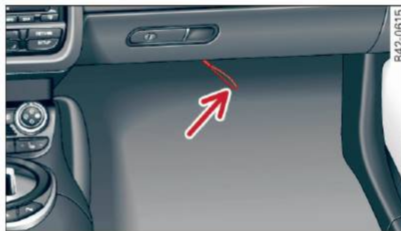
Fig. 29 Section: Emergency release
