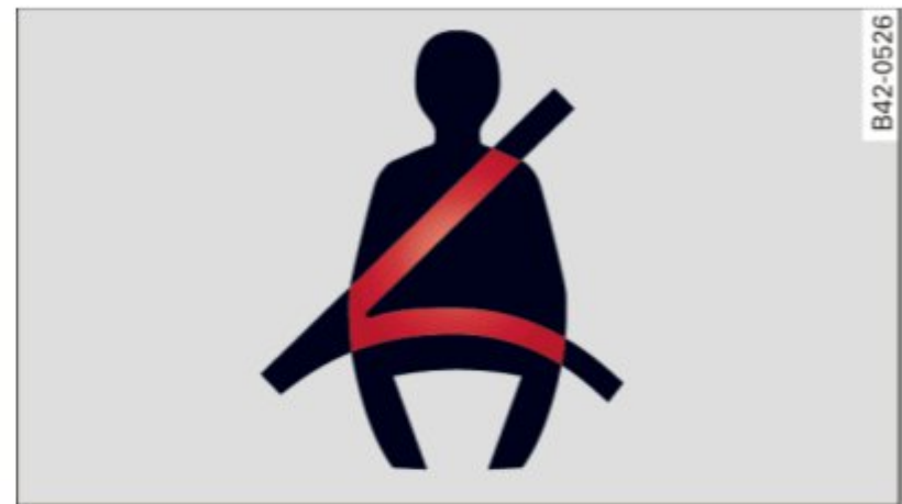
Fig. 83 Safety belt warning light in the instrument cluster - enlarged
