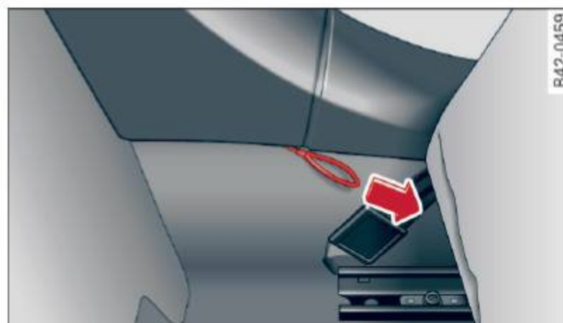
Fig. 111 Driver's footwell: emergency release loop
