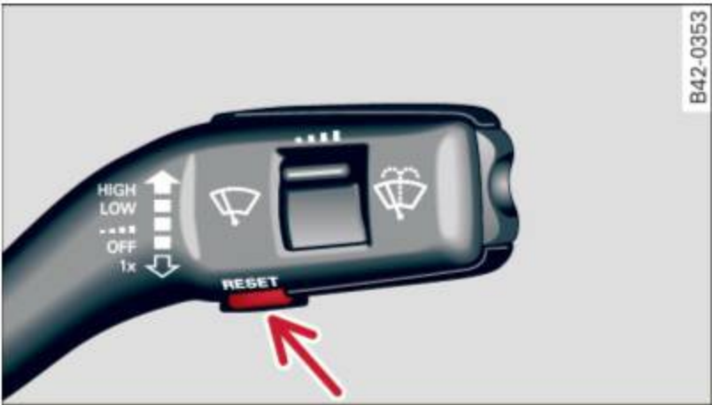
Fig. 7 Wiper lever: controls for the menu display
