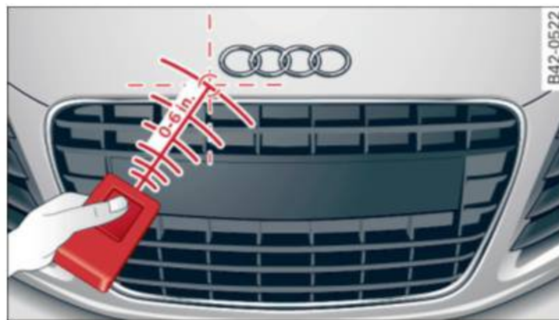
Fig. 79 Front bumper: location of transmitter unit
