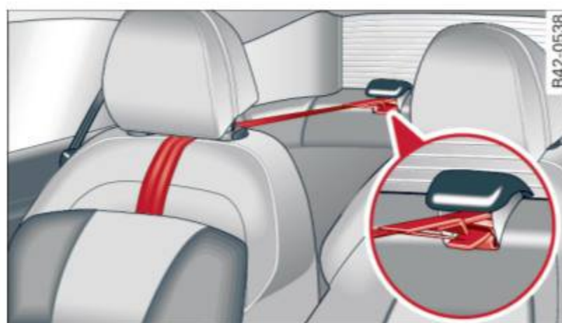
Fig. 103 Tether anchor: recess flap behind the front passenger seat
