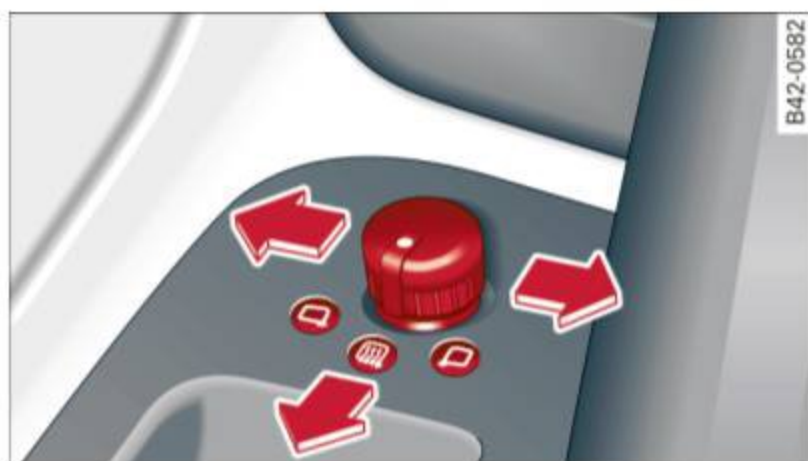
Fig. 37 Forward section of driver's armrest: power mirror controls
