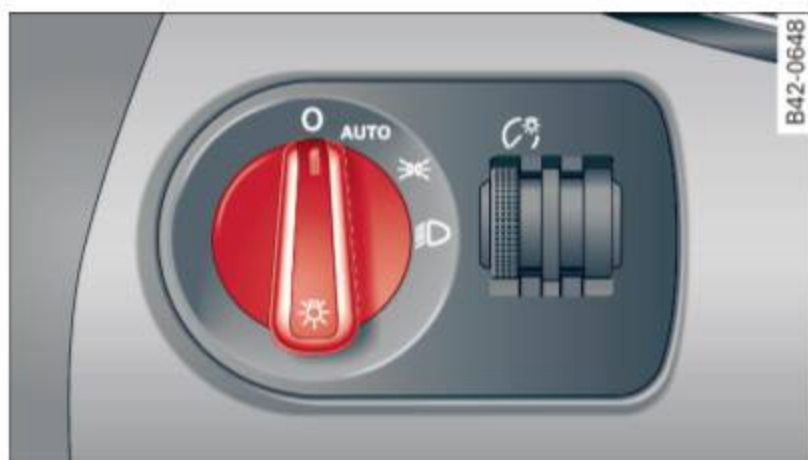
Fig. 32 Instrument panel: light switch (automatic head- and taillight control)
