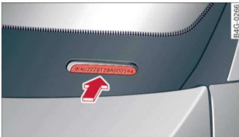
Fig. 143 Vehicle Identification Number (VIN) plate: location on driver's side dash panel
