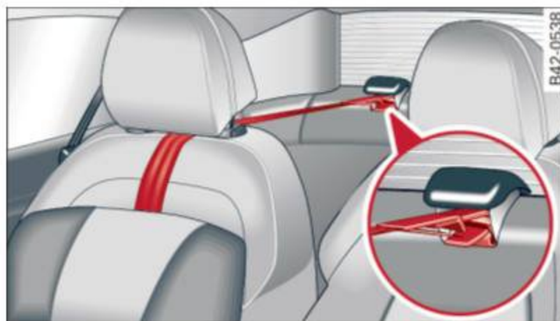
Fig. 104 Tether strap: proper routing and mounting
