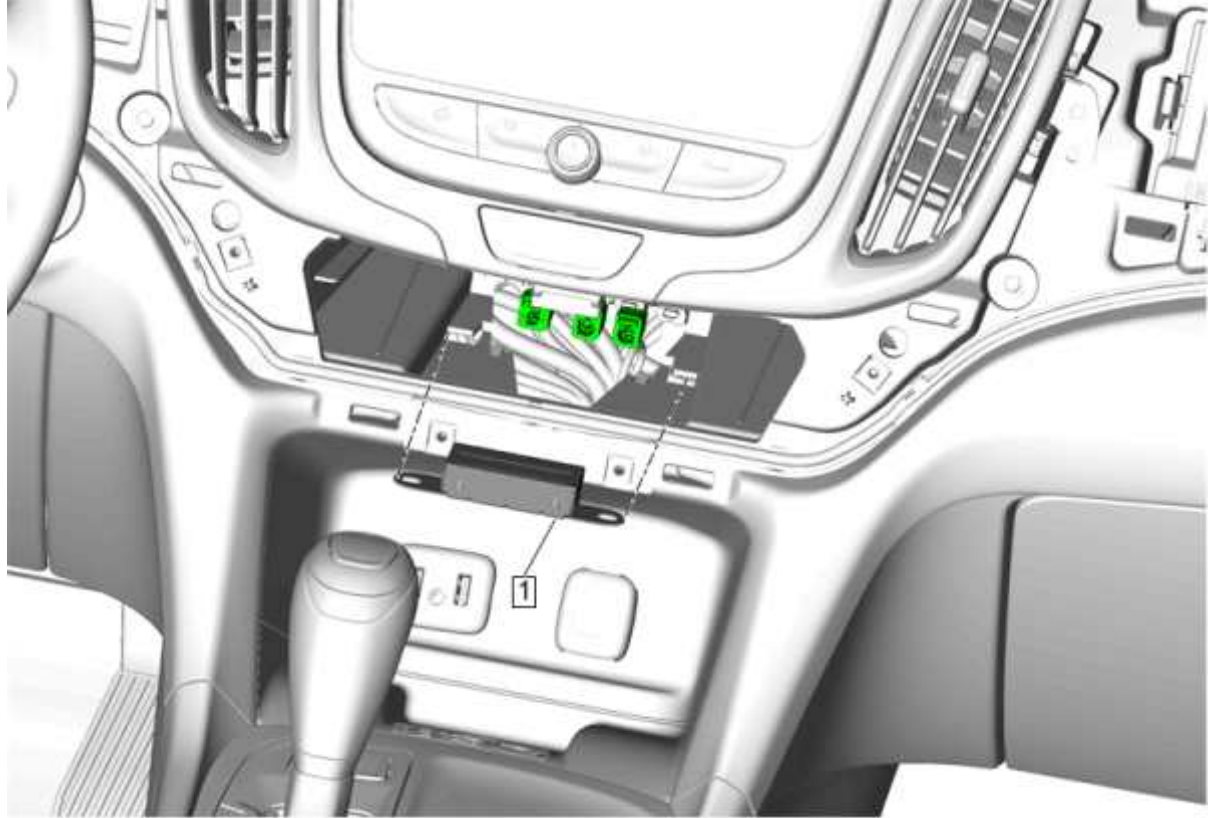
Fig. 58: Navigation Signal Splitter
