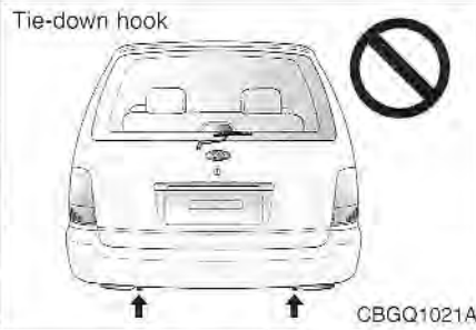
Tie-down Hook (for flatbed towing)
