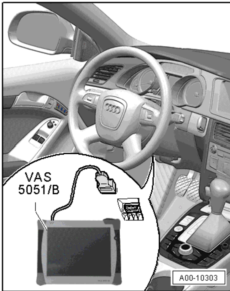
Fig. 37: Connecting Diagnostic Cable VAS 5051/5A To Diagnostic Connector Courtesy of AUDI OF AMERICA, LLC
