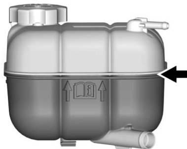
2.0L L4 and 3.0L V6 Engine Coolant Surge Tank
