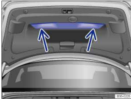
Fig. 33 Opened luggage compartment lid: Recessed grips for closing.
