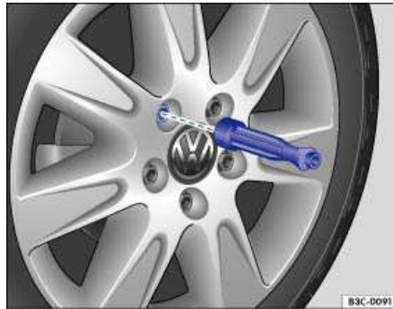
Fig. 190 Changing a wheel: Remove previously loosened wheel bolts using the screwdriver handle.
