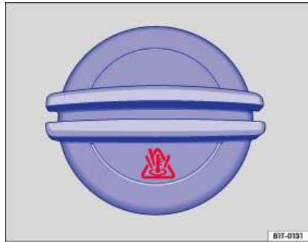
Fig. 164 Coolant expansion tank cap in the engine compartment.
