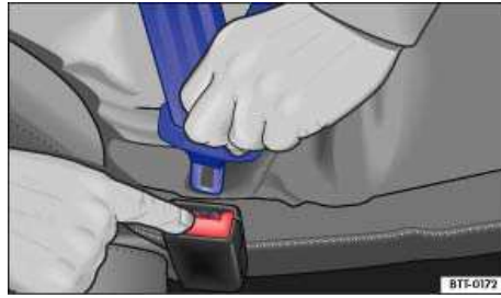
Fig. 61 Releasing the buckle tongue from the belt buckle.
