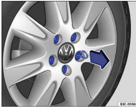
Fig. 183 Pulling cover caps off wheel bolts.
