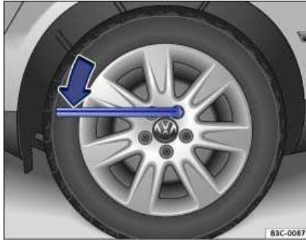
Fig. 185 Changing a wheel: Loosening wheel bolts.
