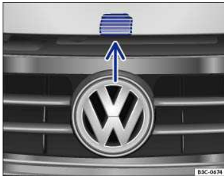
Fig. 159 Above the radiator grille: Outside engine hood release.
