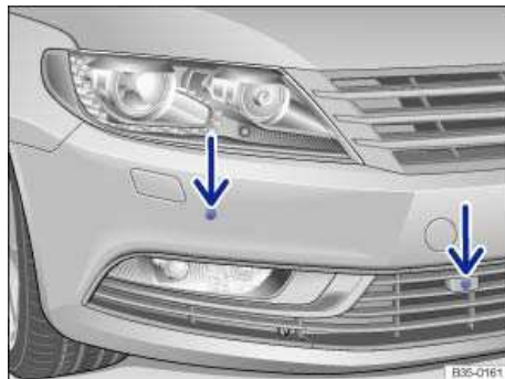
Fig. 151 In the front bumpers: Park Distance Control system sensors.
