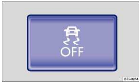
Fig. 140 In the center console: Button for switching ASR on and off manually.
