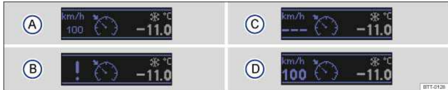
Fig. 145 In the instrument cluster display: Cruise control status indications.
