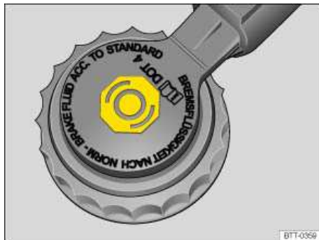
Fig. 141 In the engine compartment: Brake fluid reservoir cap.
