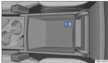
Fig. 118 In the center armrest: Location of the AUX-IN jack.
