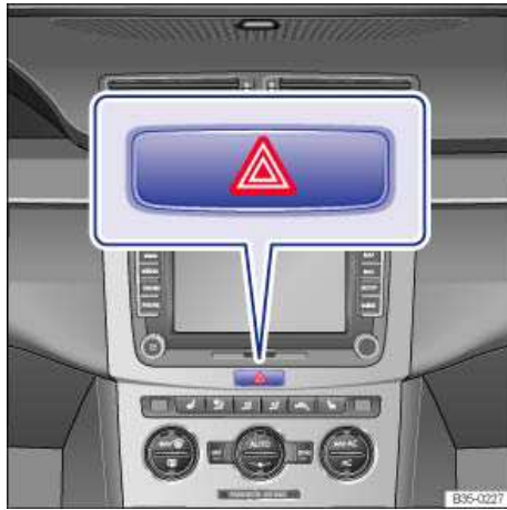
Fig. 170 In the center of the instrument panel: Button for the emergency flashers.
