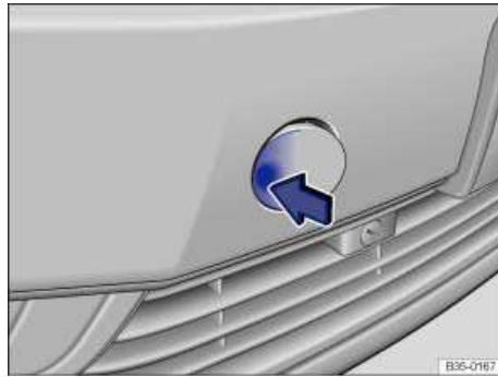
Fig. 207 In the right front bumper: Removing the cover cap.
