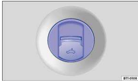
Fig. 35 In the headliner: Switch for the power sunroof.
