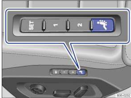
Fig. 53 On the outer side of the driver seat: Button to switch the back massage feature on and off.
