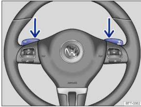
Fig. 138 Steering wheel with optional Tiptronic shift paddles.
