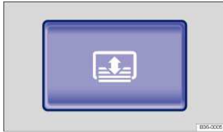
Fig. 86 In the center console: Button for the electrical sunshade on the rear window.
