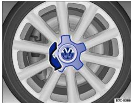
Fig. 182 Twisting the hubcap off.
