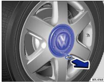
Fig. 181 Pulling the hubcap off.
