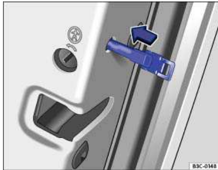
Fig. 173 Locking the vehicle using the emergency key.
