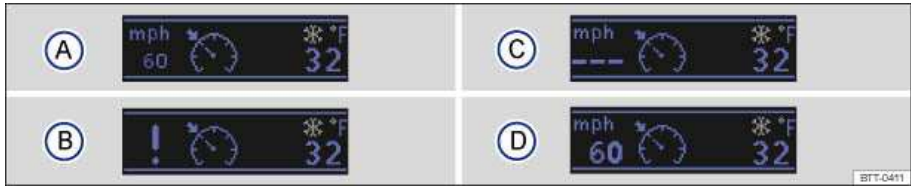
Fig. 144 In the instrument cluster display: Cruise control status indications.
