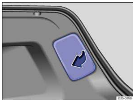
Fig. 201 In the luggage compartment lid: Removing the cover.
