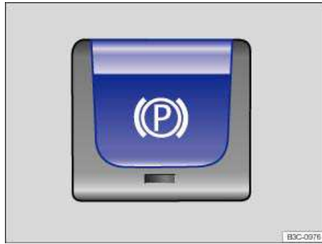
Fig. 139 In the lower section of the center console: Electronic parking brake button.
