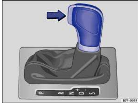
Fig. 135 Side view: Automatic transmission selector lever with shift lever release button (arrow).
