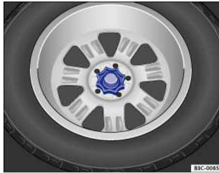
Fig. 109 In the luggage compartment: Handwheel holding spare wheel in place.
