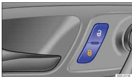
Fig. 22 In the vehicle doors: Power locking button.
