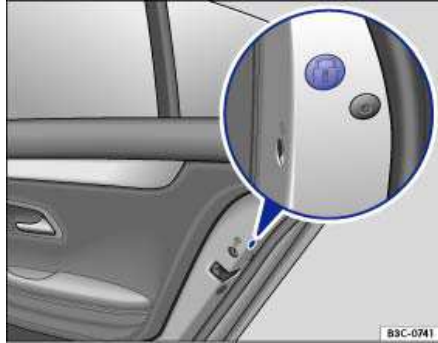
Fig. 172 On the edge of the right rear door: Emergency lock, covered by a rubber seal.
