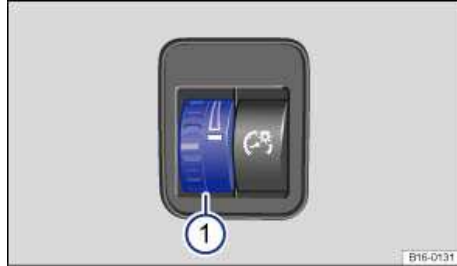
Fig. 82 To the left of the steering wheel: Thumbwheel to adjust instrument panel lighting 1.
