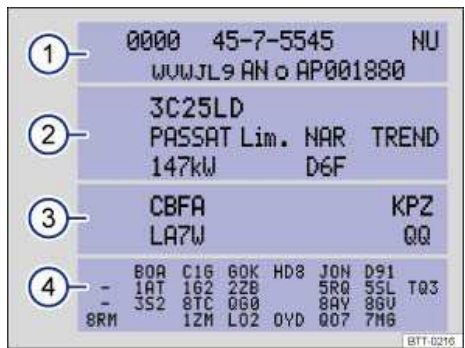
Fig. 15 Vehicle identification label: Shown in the example with engine identification code CBFA 3.
