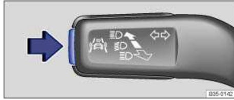
Fig. 14 In the turn signal and high beam lever: Driver assistance systems button.
