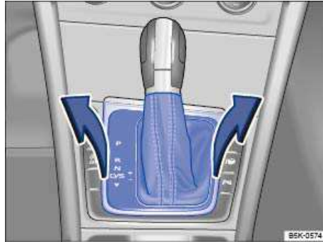
Fig. 177 Removing the selector gate cover.
