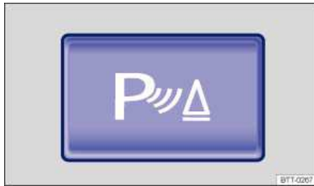
Fig. 152 In the center console: Button to switch the Park Distance Control system on or off.
