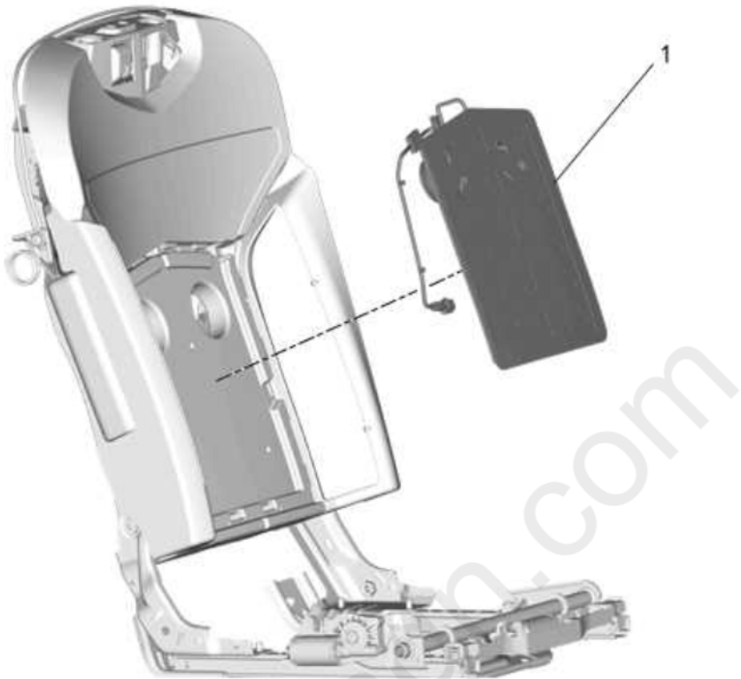
Fig. 30: Rear Seat Back Ventilation Heating and Cooling Blower Courtesy of GENERAL MOTORS COMPANY
