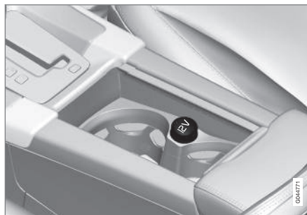
12 V socket in tunnel console, front seat.
