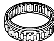
ONE-WAY CLUTCH Inspect for damage or faulty movement.
